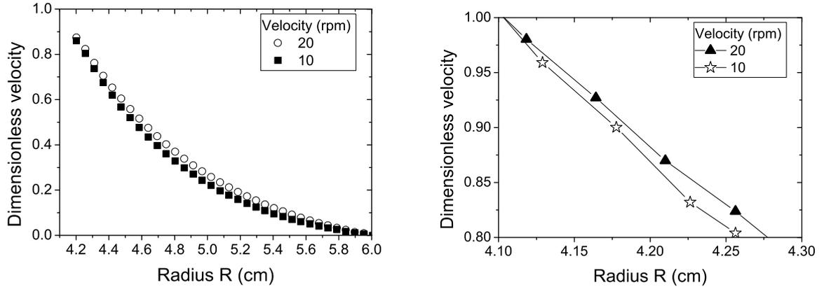
FIG. 6: a) Dimensionless velocity profiles for the steady flows of a  $6.5\mu\text{m}$  adhesive emulsion, for a 10 and a 20 rpm rotational velocity. b) Dimensionless velocity profiles expected near the walls at 10 and 20 rpm; the velocities are computed thanks to the local shear rate measurements performed at 50 rpm.
