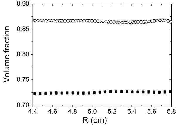
FIG. 1: Concentration profiles observed within the gap of a Couette geometry after shearing a  $0.3\mu\text{m}$  adhesive emulsion for 10000 revs (squares), and a  $40\mu\text{m}$  non-adhesive emulsion for 20000 revs (open circles).
