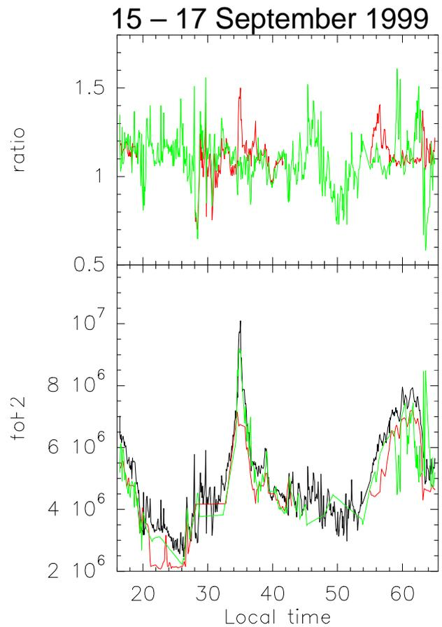
**Fig. 2.** *foF2* comparison between the IS radar data (black), the Dynasonde (red) and the DGS (green). The top panel shows the ratio between the ionosonde-*foF2* data and the IS-*foF2* data in the same colour scheme.
