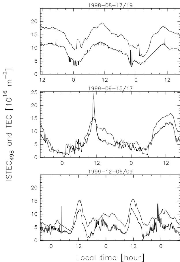
**Fig. 7.** Comparison between the TECs derived from the GPS stations (thin lines) and the calibrated ISTEC<sub>498</sub> derived from the EISCAT measurements (bold lines). Only the three corrected periods are shown.
