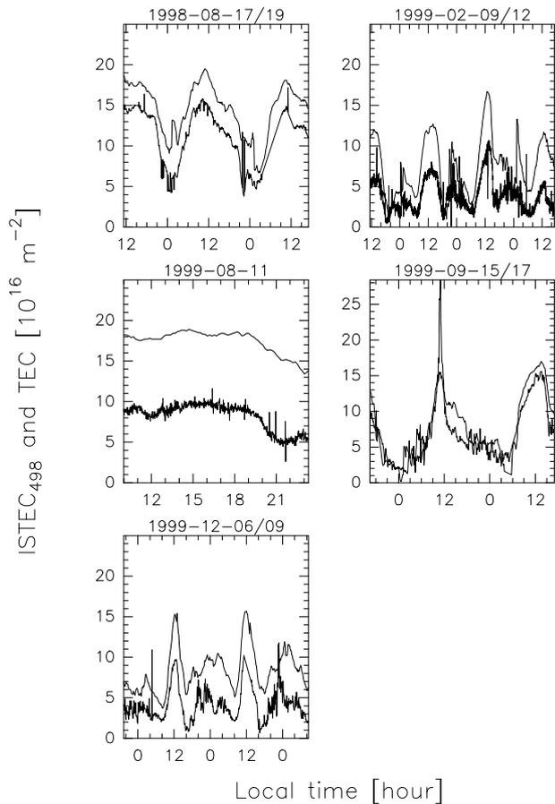
**Fig. 1.** Comparison between GPS TEC (thin lines) and the ISTEC<sub>498</sub> derived from the uncalibrated EISCAT measurements (bold lines).
