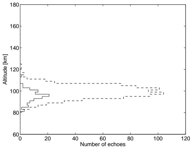
**Fig. 3.** Altitude distribution of head echoes from the August campaign 1993 recorded with the UHF radar (solid line) and by the VHF radar (dashed line). Note the difference in rate scale from the previous figure.
