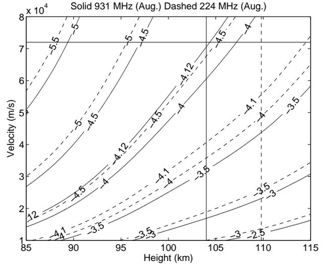
**Fig. 10.** As Fig. 9, but showing UHF and VHF (224 MHz) critical density altitudes in an August atmosphere. Dashed lines are VHF, solid lines are UHF. The vertical lines indicate the corresponding cutoff altitude.
