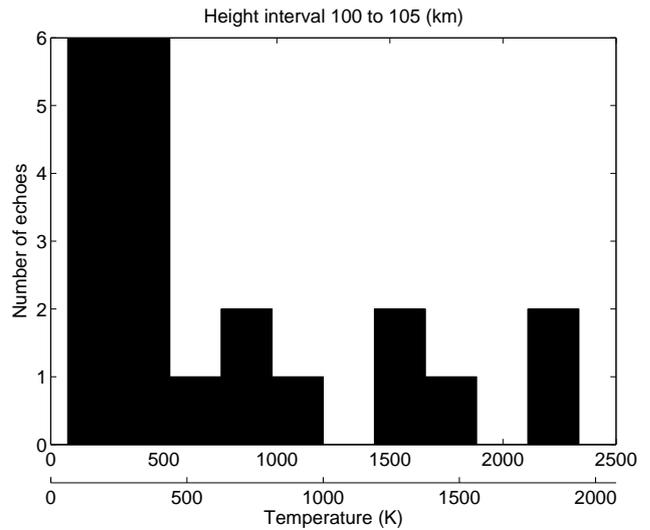
**Fig. 6.** The effect of the range factor of the scattering from the August UHF target temperature distribution over 100–105 km altitude range (the upper axis). The lower axis gives the equivalent noise temperature as if the same distribution had been displaced 5 km upwards.
