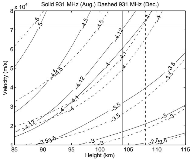
**Fig. 9.** Showing the altitude at which the ionisation produced by a meteor of a given size first reaches critical density at the EISCAT UHF frequency, 930 MHz, with  $\log$  (meteor radius in meters) as a parameter. Height is related to atmospheric density through the MSISE-90 model. Solid lines represent an August atmosphere and dashed lines a December atmosphere. The vertical lines indicate the corresponding cutoff altitudes.
