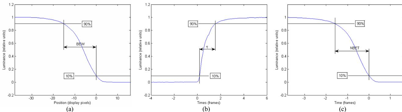
Figure 2 - Illustration of measurement performed for a transition from  $N_s = 0$  to  $N_f = 255$ : blurred edge profile obtained by spatial measurement of an edge moving at  $V = 10$  pixels per frame (a), temporal step-response (b) and blurred edge profile obtained from the step-response (c).
