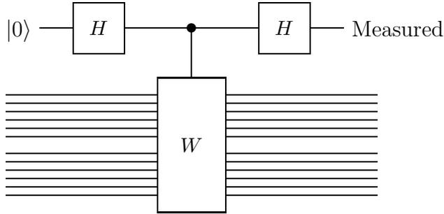
Figure 1: A circuit implementing the swap test.
