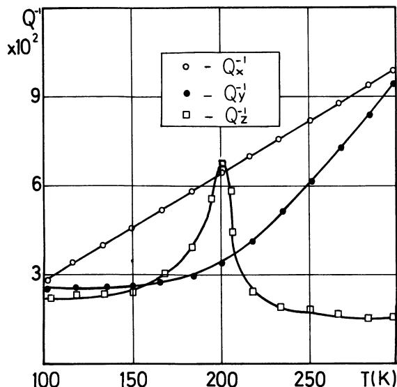
Fig. 3. — Temperature dependence of internal friction  $Q_x^{-1}$ ,  $Q_y^{-1}$  and  $Q_z^{-1}$  in NaKSO<sub>4</sub> crystals.
