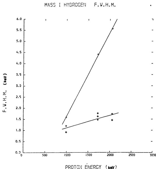
FIG. 3. — Measured full width at half maximum of various  $^{27}\text{Al}$  (p,  $\gamma$ ) resonances. The target thickness was not more than 100 eV at 1 MeV. The lower curve is a composite of many measurements over several months of normal operation. The higher curve was measured when rectifiers in the oscillator power supply were faulty.
