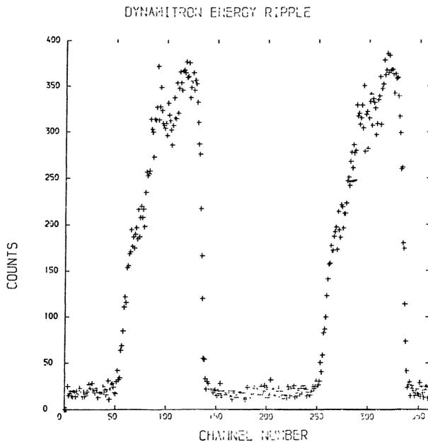
FIG. 4. — Yield from the 992 KeV  $^{27}\text{Al}$  ( $p, \gamma$ ) resonance measured in time correlation with 50 Hz mains frequency. The time axis calibration is 100  $\mu\text{s}$  per channel and the figure covers nearly two full cycles. The strong time correlation is clear.
