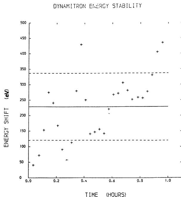
FIG. 2. — The energy shift, as a function of time, of the Dynamitron measured by observing the change in count rate on the very sharp leading edge of the 992 KeV  $^{27}\text{Al}$  (p,  $\gamma$ ) resonance.
