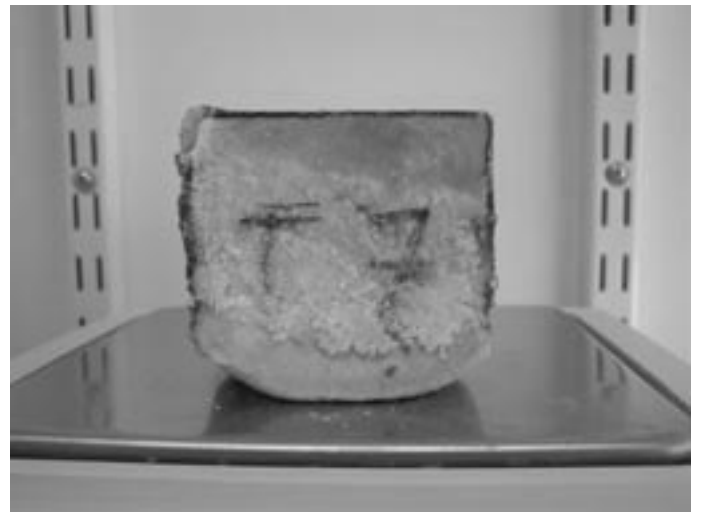
Figure 2. Picture of a 7x7x7 cm 3 sample with the four lower corners damaged (SF, capillary imbibition & remobilisation after 7 cycles).
