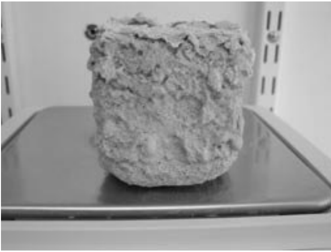
Figure 9a. Picture of a 7 \times 7 \times 7 \text{ cm}^3 non-isolated sample of FL after cycle 12.
