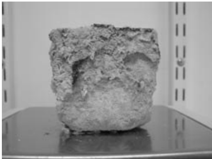
Figure 4b. Picture of a 7 \times 7 \times 7 \text{ cm}^3 sample of FL after 6 cycles of capillary imbibition & remobilisation.
