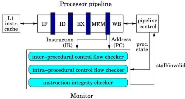
Fig. 2. Proposed hardware-assisted monitoring architecture: Conceptual block diagram
