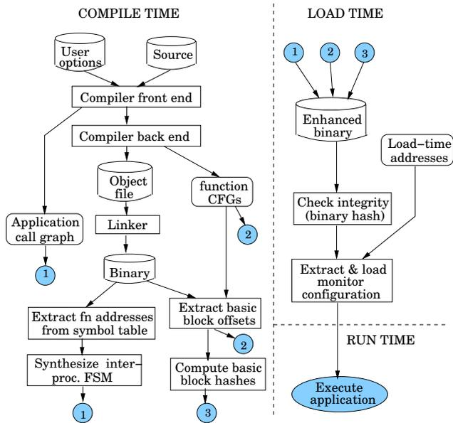
Fig. 4. Design flow for hardware-assisted run-time monitoring
