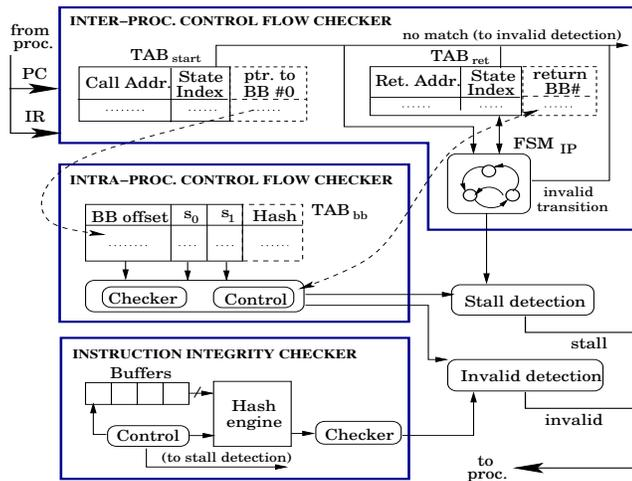
Fig. 3. Architectural details of the run-time monitor
