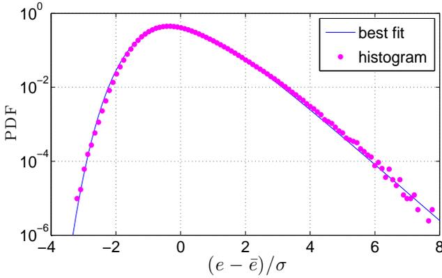
Fig. 4: A histogram of the centered and normalised induced voltage  $x(t) = (e(t) - \bar{e})/\sigma$  at fixed current  $I$  is plotted in semi-log axis (dots). The fitting is performed with a GG distribution (line). The best fit is obtained for  $a = 2.5$ .
