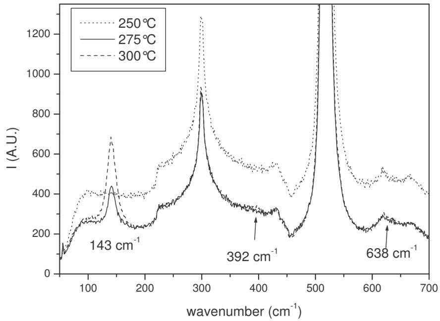
Figure 1 Raman spectra of  $\text{TiO}_2$  samples deposited from  $\text{Ti}(\text{OiPr})_2(\text{thd})_2$ . Peaks associated to anatase are indicated
