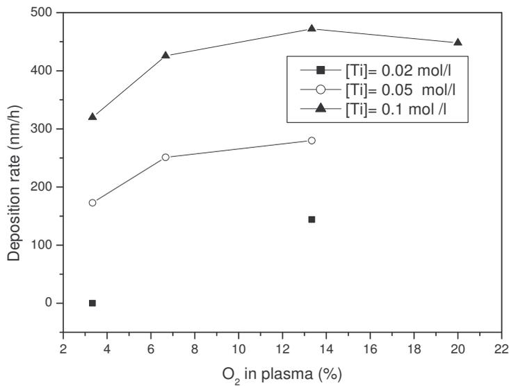
Figure 4. Variation of the deposition rate as a function of oxygen content in plasma for several Ti concentrations of TiO(acac)<sub>2</sub> in solution
