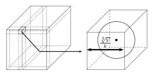
Split the cube of volume V into  $k^3$  subcubes,  $\mathcal{R}_1, \dots, \mathcal{R}_{k^3}$  of equal volume. Each of these sub-cubes has side  $\sqrt[3]{V}/k$ . Choose k such that a sphere of radius  $R_{\text{TRANS}}$  can entirely fit inside a sub-cube  $\mathcal{R}_i$  (cf. figures).
