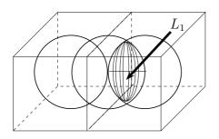
The lens-shaped region, here denoted  $L_1$ , represents the intersection of two spheres of radius  $R_{TRANS}$  and whose centers are at distance  $R_{TRANS}$ . A bit of trigonometry shows that the volume of such intersection is given by  $\frac{5 \pi R_{TRANS}^3}{12}$ .
