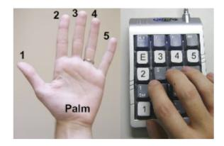
Figure 10: Five-key: A technique using sequences of short and long keypresses to enter any letter with just five keyboard keys (Szentgyorgyi and Lank, 2007)
