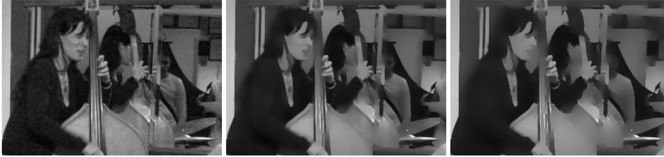
Figure 4.2: **Perona-Malik diffusion**: from left to right, original image, after 50 iterations and after 200 iterations
