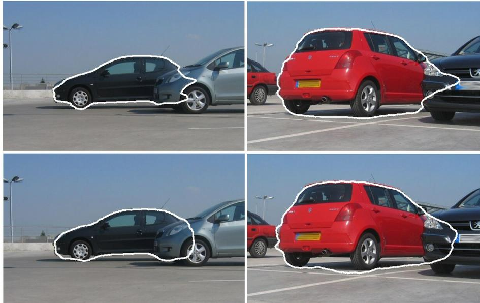
Figure 8.10: **Segmentation with shape priors (car manifold), attracting force # 3** - Segmentation of a Peugeot 206 (left) and a Suzuki Swift (right). First row: Segmentation with data term only. Second row: segmentation with our shape prior. The embedding of the final shape is denoted by a blue cross and a green cross respectively for the Peugeot 206 and the Suzuki Swift in Figure 8.9
