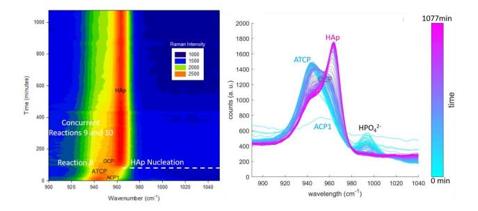
Figure 4. Time-lapse Raman spectroscopy monitoring of the formation of hydroxyapatite (HAp) in experiment 3 (Table 1). (left) Raw data Raman spectra between 0 and 1077 minutes showing the transformation of ATCP into OCP (reaction 8 in the text) and the synchronous transformations of OCP into hydroxyapatite (reaction 9 in the text) and ATCP into hydroxyapatite (reaction 10 in the text). (right) Time-lapse evolution of the main peaks used for deconvolution fitting.
