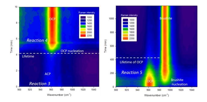
Figure 2. Time-lapse Raman spectroscopy monitoring of the formation of brushite in experiment 2 (Table 1). (left) Raw data Raman spectra between 0 and 10 minutes showing the formation of ACP (reaction 3 in the text) and the nucleation time of OCP (reaction 4 in the text). (right) Raw data Raman spectra from 0 to 1200 minutes showing the transformation of OCP into brushite (reaction 5 in the text).
