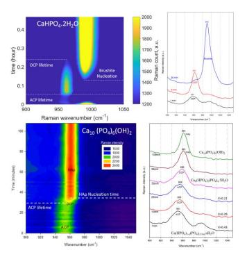
**Synopsis:** The nucleation of brushite and hydroxyapatite was monitored in real-time by Raman spectroscopy at 25 °C. For both minerals, amorphous calcium phosphate  $(Ca(HPO_4)_{1-x}(PO_4)_{(2/3)x}.nH_2O)$  with different Raman signature instantaneously formed in the initial solution. Then, the amorphous phases transform into OCP, a crystalline transient phase. Finally, OCP transforms into brushite micro-crystals or into hydroxyapatite nanocrystals.
