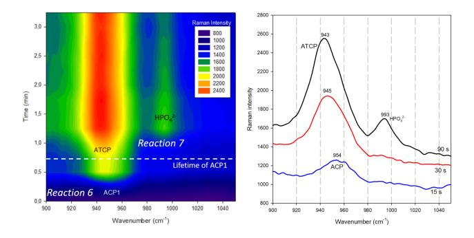
Figure 3. Time-lapse Raman spectroscopy monitoring of the formation of hydroxyapatite (HAp) in experiment 3 (Table 1). (left) Raw data Raman spectra between 0 and 3 minutes indicating the formation of ACP1 (reaction 6 in the text) and the transformation of ACP1 intoATCP (reaction 7 in the text). (right) Three raw data Raman spectra at 15, 30 and 90s showing a fast shift of the position of the Raman peak of amorphous phases from 954 to 943cm<sup>-1</sup>.
