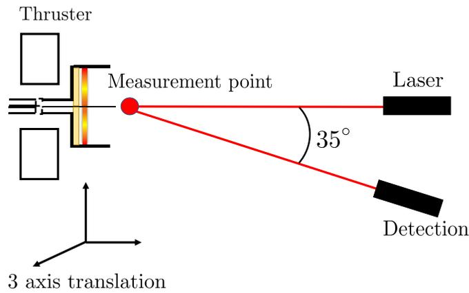
Figure 3: Schematic of optical LIF setup inside the vacuum chamber
