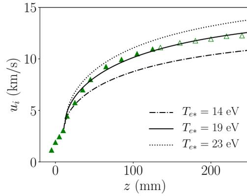
Figure 13: Experimental ion velocity curve  $u_i(z)$  with the model predictions at different values of  $T_{e^*}$  for 2 sccm.
