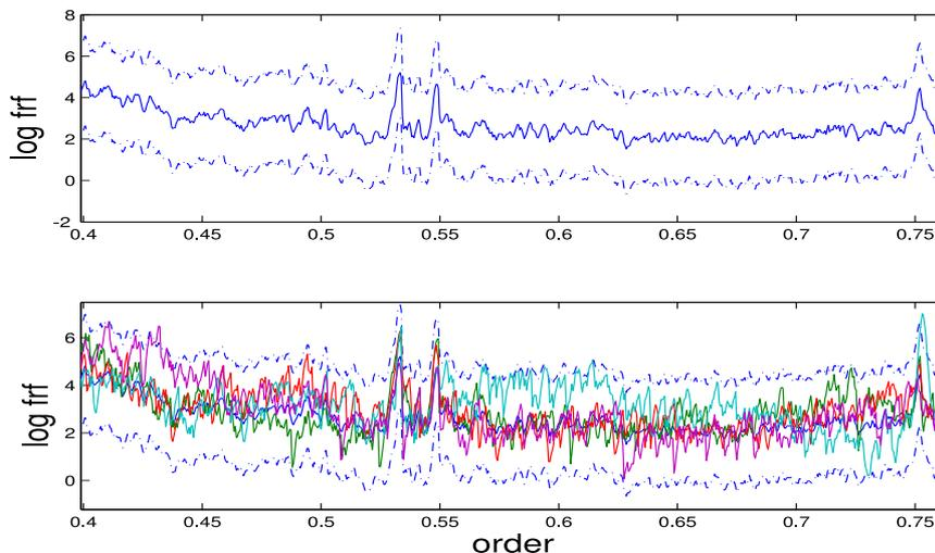
Figure 4: FRF in the order domain (top) predicted mean and associated confidence interval (bottom) superimposed FRF of all engines.
