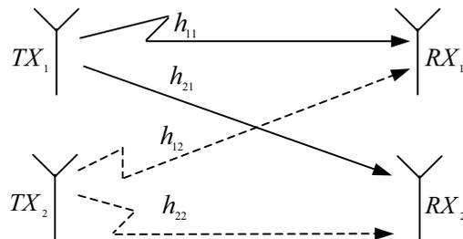
Figure 2. Channel Model for MIMO  $2 \times 2$
