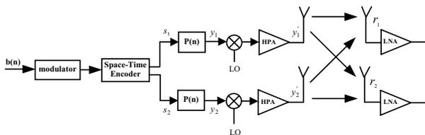
Figure 3. Communication system using the Alamouti scheme
