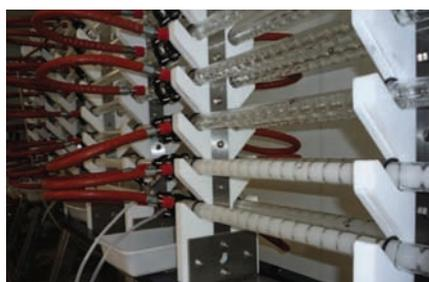
Suitable to perform **liquid-liquid dispersion** of controlled mean droplet size
