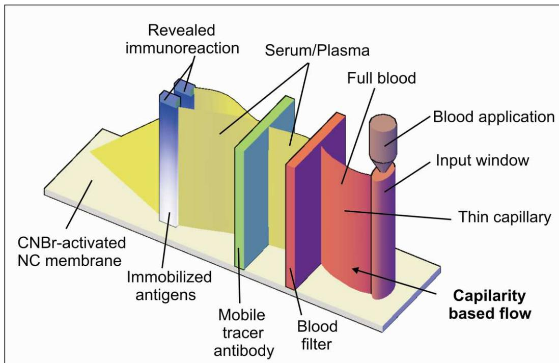
Fig. 13 Detailed view of internal composition of testing zone in a miniaturized diagnostic device. CNBr-activated: cyanogen bromide (CNBr)-activated, NC: nitrocellulose.
