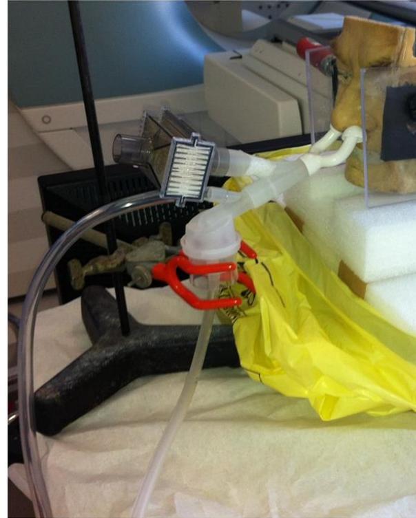
Supplementary Information: Experimental set-up for nebulization. A and B corresponds to photography of the set-up in the Nuclear Medicin department (CHU Saint-Etienne).
