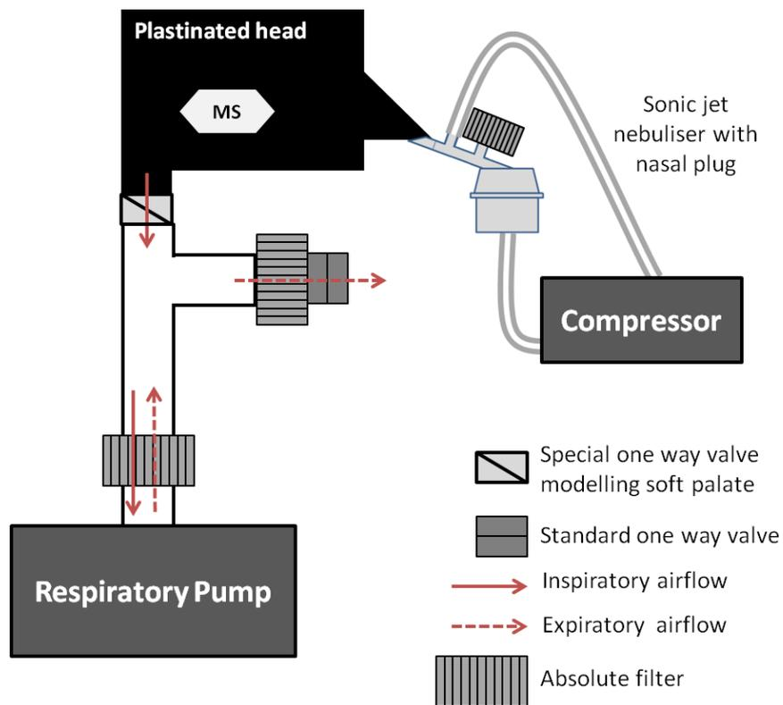
Figure 1: Schematical experimental set-up for nebulization simulating an inspiration by the nose and exhalation through the mouth thanks to the respiratory pump.
