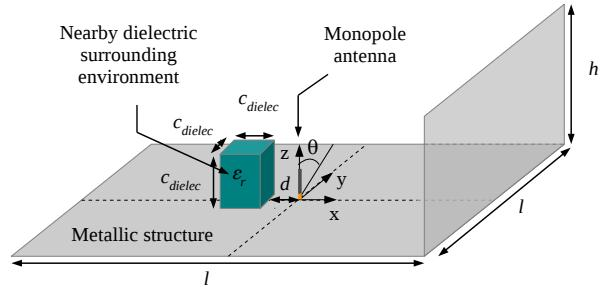
Fig. 1. Antenna mounted on a metallic structure.  $l = 3.9 \text{ m} = 13 \lambda_{1\text{GHz}}$ ,  $h = 1.15 \text{ m} = 3.83 \lambda_{1\text{GHz}}$ ,  $d = 0.15 \text{ m} = 0.5 \lambda_{1\text{GHz}}$ ,  $C_{dielec} = 0.18 \text{ m} = 0.6 \lambda_{1\text{GHz}}$ ,  $\epsilon_r = 10$
