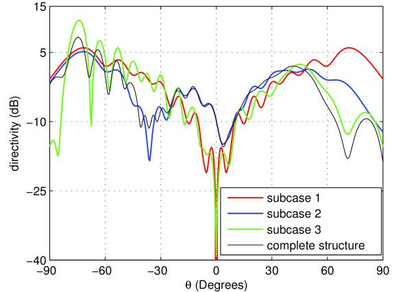
Fig. 4. Far-field results ( $E_\theta$ ) in the (x0z) plane at 1 GHz.
