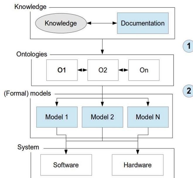
Fig. 4. Ontologies in the formalised development of safety critical systems
