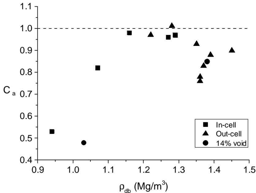
Figure 6. Anisotropy coefficient variation with bentonite dry density for different test conditions
