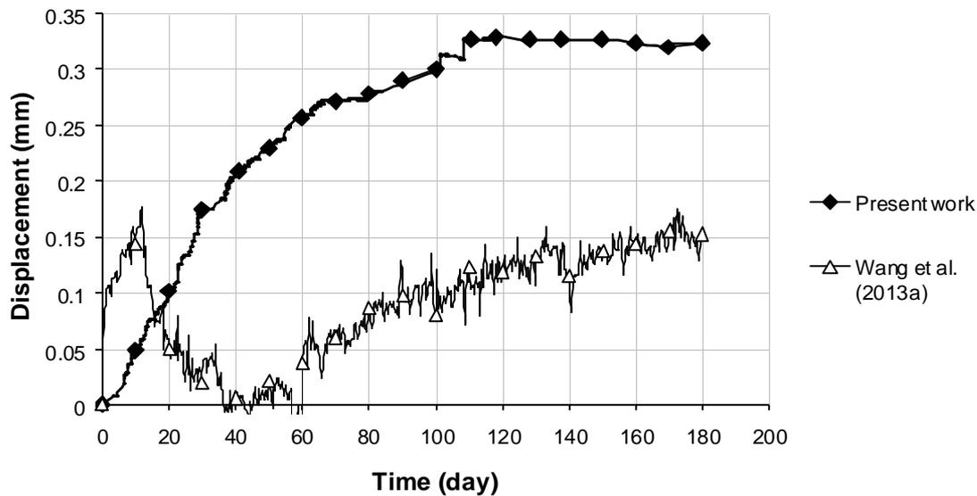
Figure 10. Evolution of the piston's displacement over time in the present work and in the work of Wang et al. (2013a).
