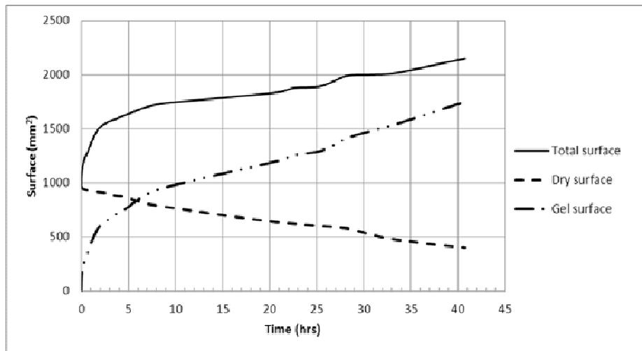
Figure 6 Variation of the total surface, dry surface and gel surface with time for a bentonite-sand disk having a density of 1.97 Mg/m<sup>3</sup>.
