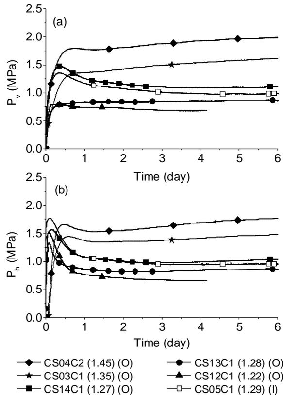
**Figure 3. Kinetics of the axial (a) and radial (b) swelling pressure for different bentonite dry densities; The letters O and I in the legend refer to the method of sample preparation: Out-cell and In-cell, respectively.**
