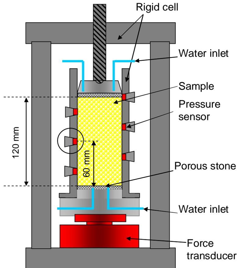
Figure 6. Layout of the swelling pressure laboratory test cell with positions of the sensors.
