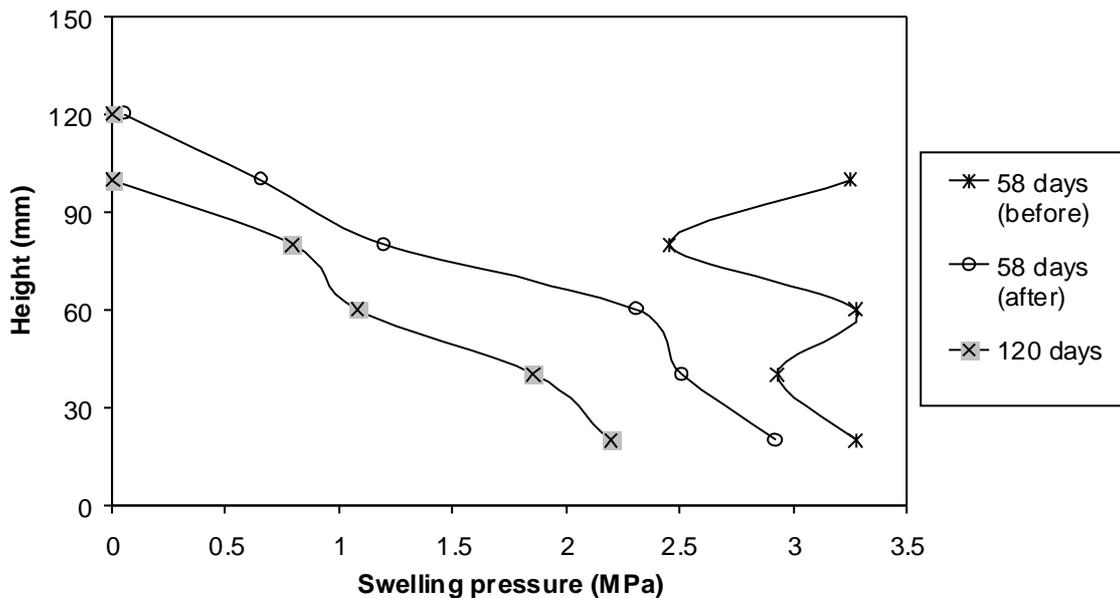
Figure 18. Swelling pressure profiles at the start of step 2 (at 58 days, just before and after the piston release) and at the current stage of test (at 120 days).
