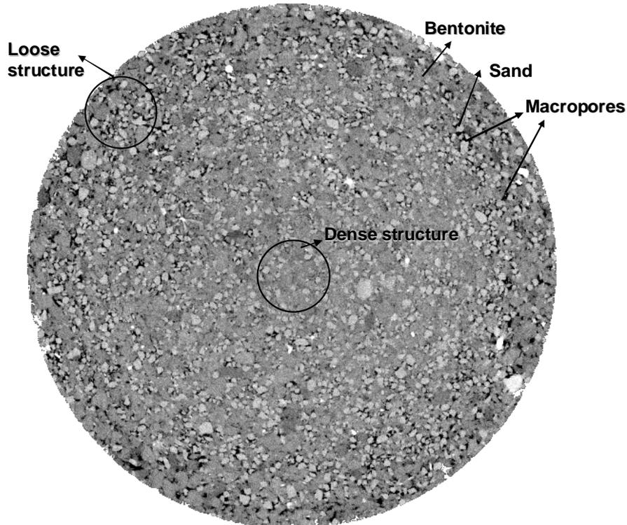
**Figure 4. A typical radial  $\mu$ CT cross-section of the compacted bentonite/sand mixture sample.**
