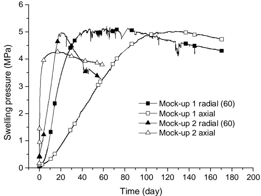
**Figure 11. Evolution of the small scale radial and axial swelling pressures in Mock-up 1 and Mock-up 2 tests.**
