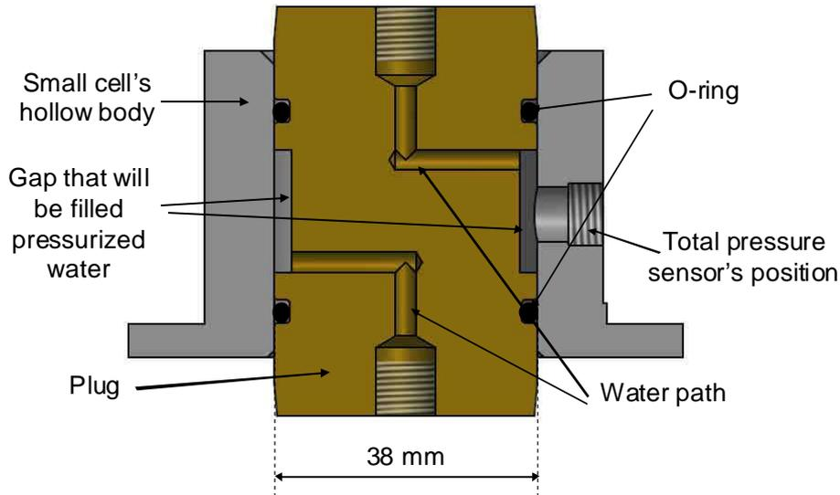
**Figure 6. Calibration plug for total pressure sensors inserted in the small cell.**
