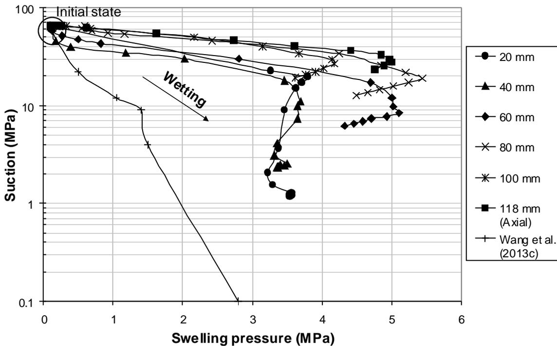
Figure 15. Suction versus swelling pressure for different infiltration lengths.
