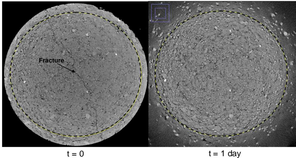
**Figure 6. Fracture closure after 1 day of hydration. The circular line outlines the unsaturated part after 1 day and its position is reported in the initial state.**
