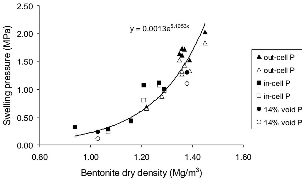
**Figure 5. Variation of vertical and horizontal swelling pressures with bentonite dry density under different test conditions**
