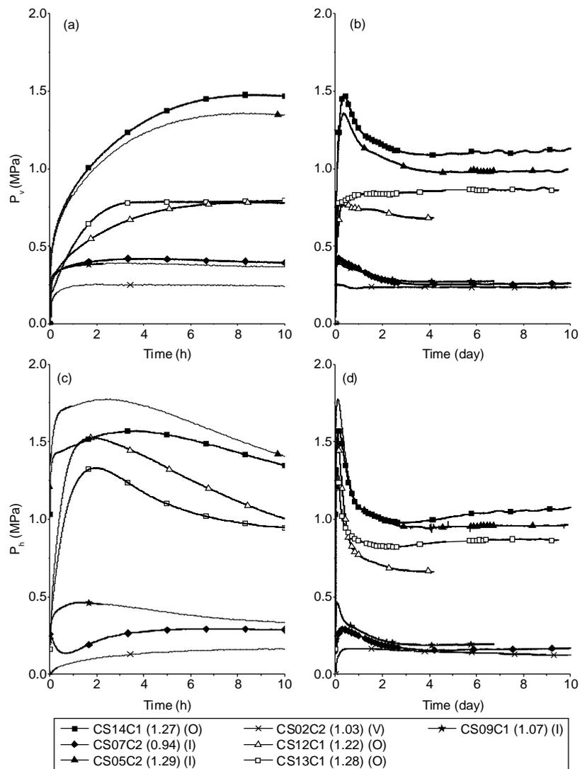
**Figure 4. Kinetics of vertical and horizontal swelling pressure for low bentonite dry densities (a,c) at the first 10 hours and (b,d) for the whole duration of test; The letters O, I and V in the legend refer to the method of sample preparation: Out-cell, In-cell and with 14% Void respectively.**
