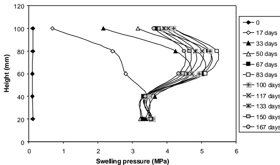
Figure 5 Swelling pressure profiles evolution at a time interval of 17 days from Mock-up 1.
