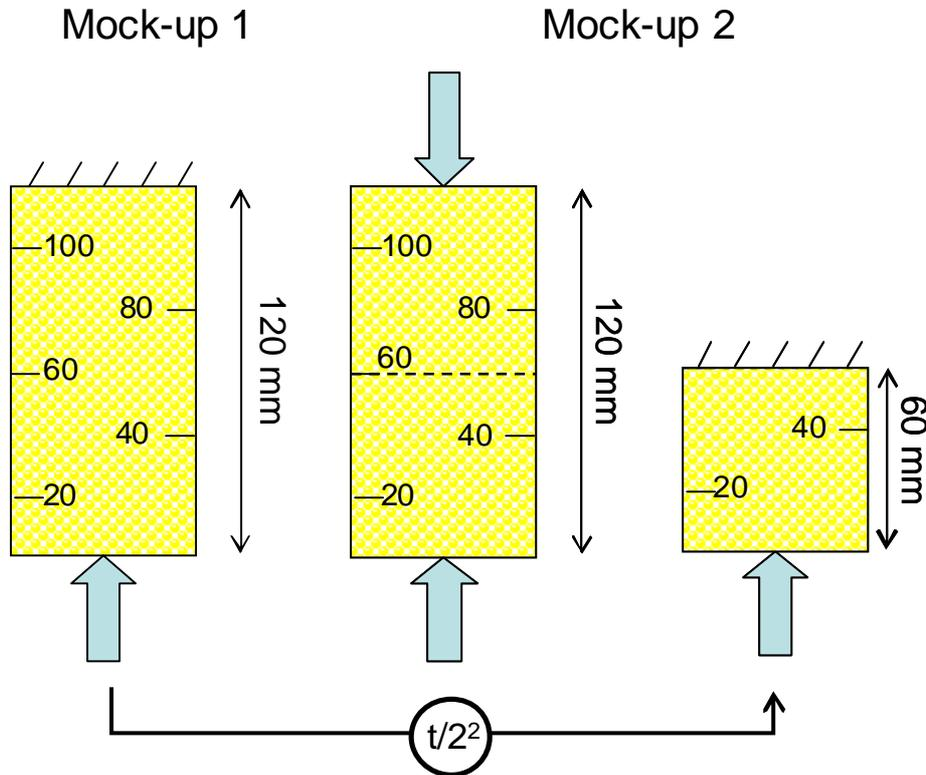
Figure 9. Sketch of the samples with their respective boundary conditions in both tests and after considering the symmetry plan in Mock-up 2.
