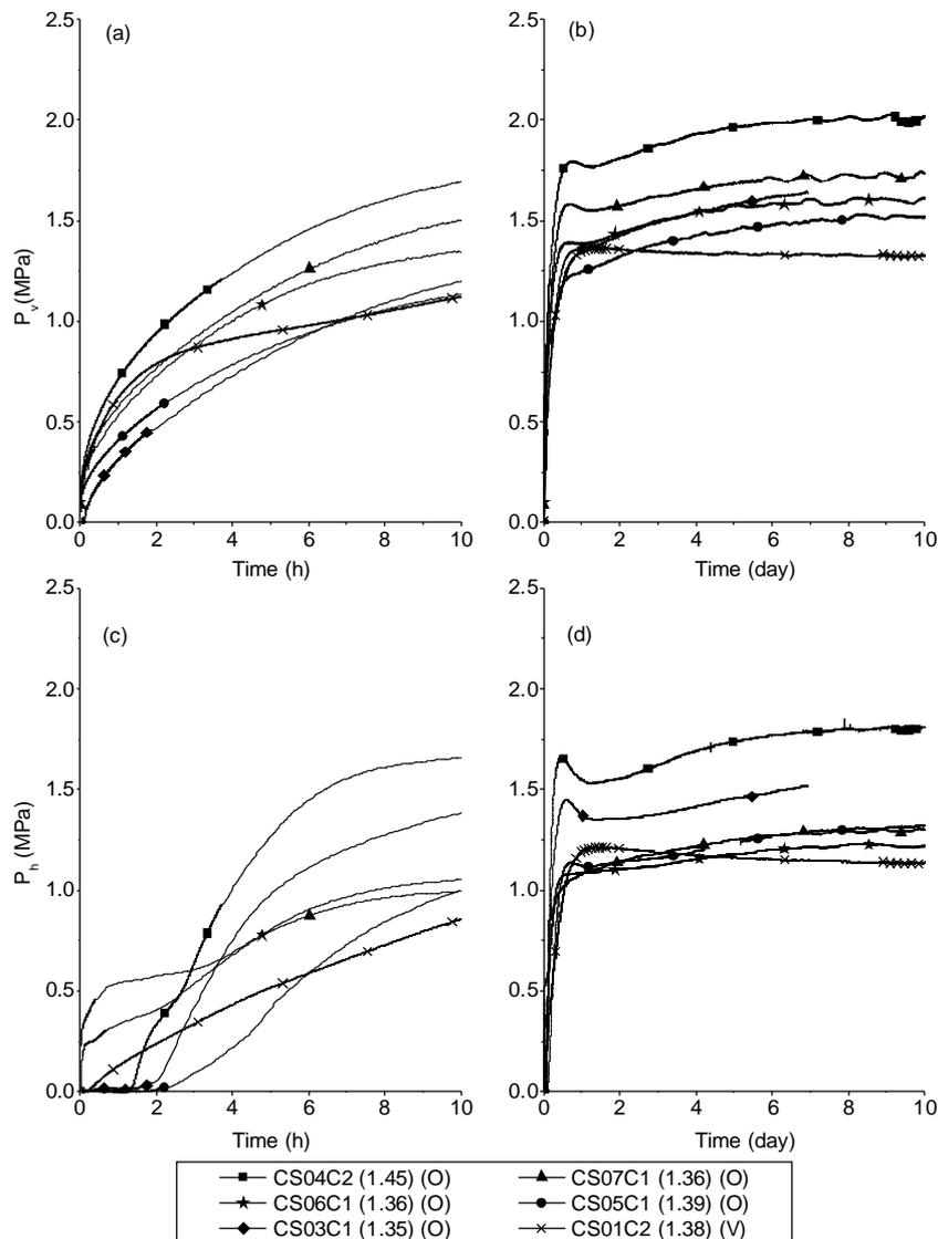
**Figure 3. Kinetics of vertical and horizontal swelling pressure (a,c) at the first 10 hours and (b,d) for the whole duration of test in the case of high bentonite dry densities; The letters O, I and V in the legend refer to the method of sample preparation: Out-cell, In-cell and with 14% Void, respectively.**
