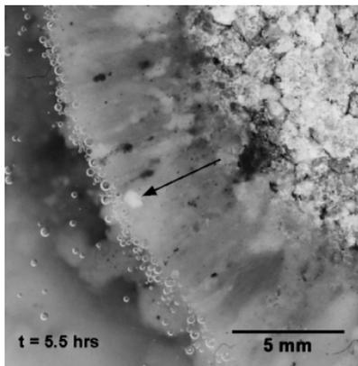
**Figure 7** A sand grain pushed radially in the gel formation.
