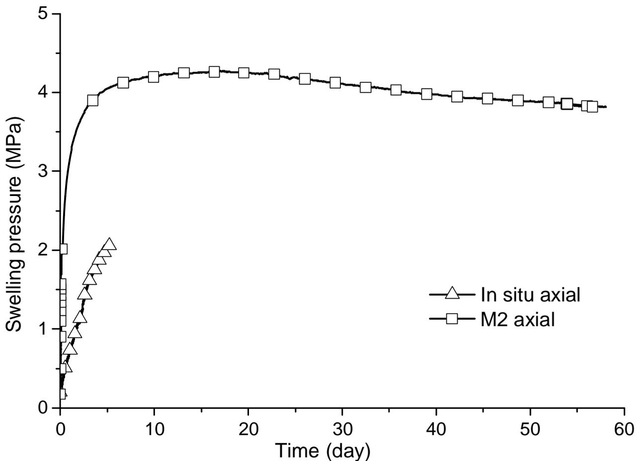
Figure 12. Comparison of the axial swelling pressure measurement at 0 mm distance to the wetting source between the in situ test and Mock-up 2.
