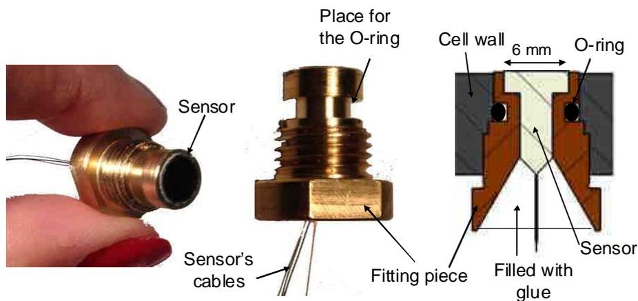
Figure 5. Total pressure sensor's fitting piece.
