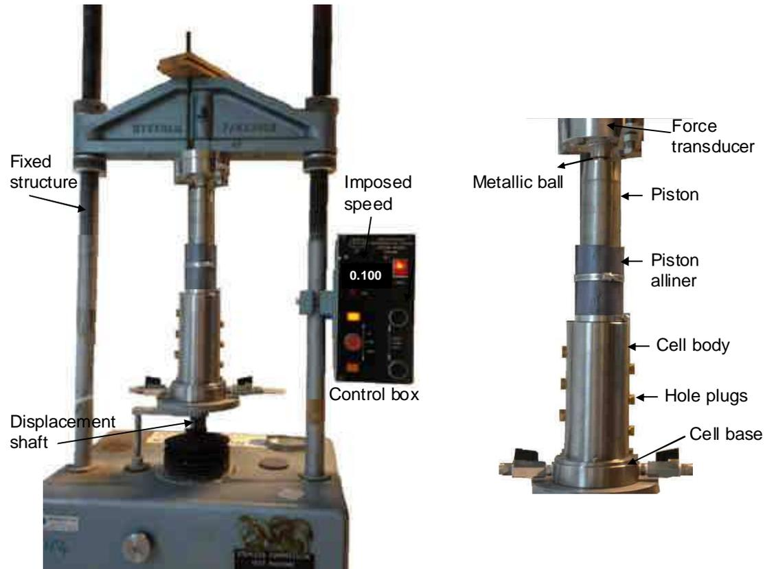
**Figure 8. Sample compaction in the mechanical press.**
