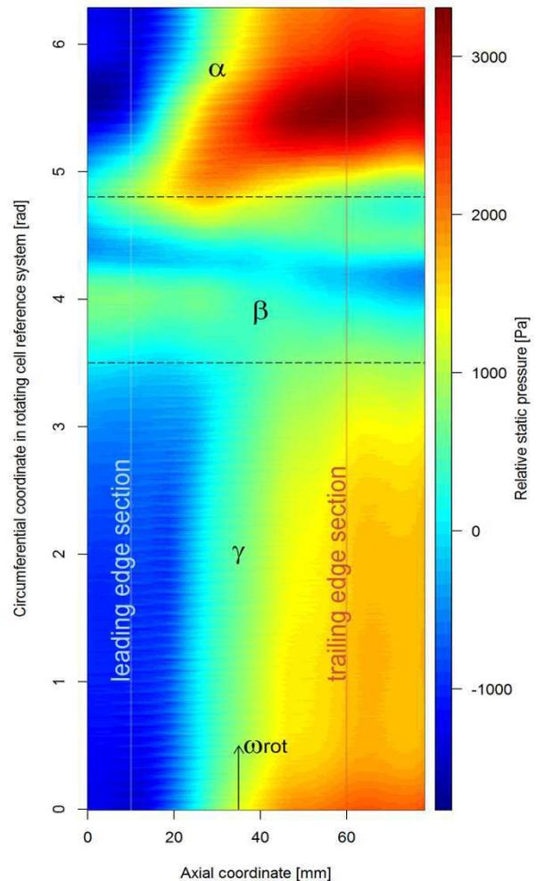
Figure 7 Average casing pressure field during rotating stall
