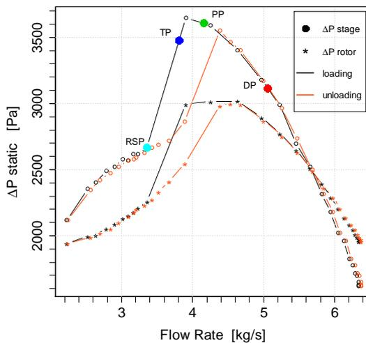
Figure 3 Performance characteristics of the compressor at 3200 rpm
