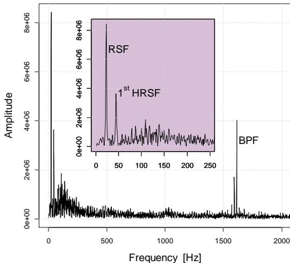
Figure 6 Frequency domain analysis,  $q_{RSP}=3.35\text{kg/s}$ , transducer location  $0\text{mm}-0^\circ$
