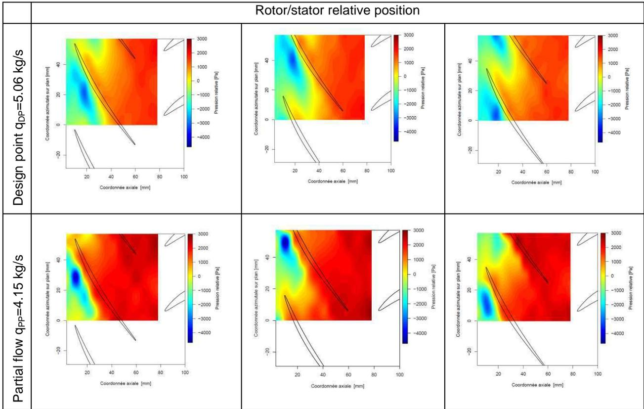
Figure 4 Phase-averaged pressure fields for normal operating conditions
