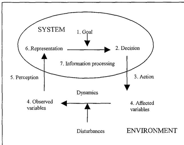
Figure 2: basic components of a control system
