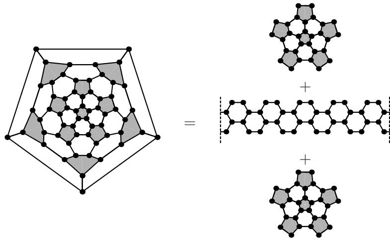
Figure 2: The buckyball is the first nanotube of type  $(5, 5)$ .
