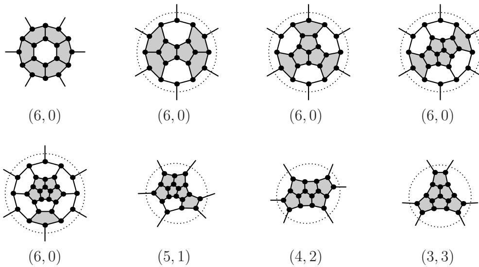
Figure 8: The caps of  $(p_1, p_2)$ -nanotubes, where  $p_1 + p_2 = 6$ .
