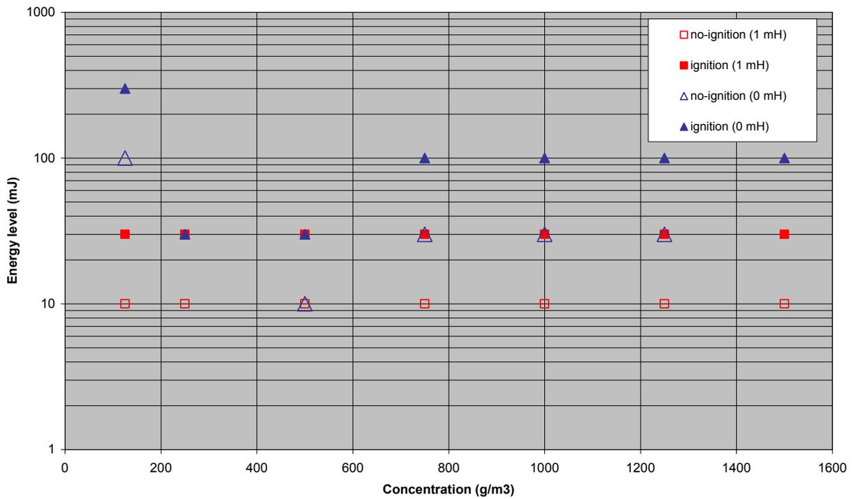
Figure 7: Comparison of MIE evolution with average particle concentration for lycopodium dust on MIKE 3 explosion tube with and without inductance. Average particle concentration is based on the amount of dust placed in the bottom cup prior to the test and the volume of the explosion tube (delay between dispersion and sparkover: 180 ms).
