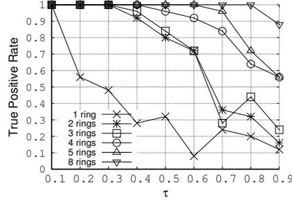
Fig. 9. Effect of the Score threshold  $\tau$  on the TPR
