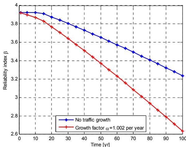
Figure 7. Influence of traffic growth on structural resistance
