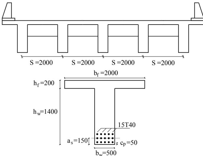
Figure 5. Cross-section of transverse bridge and T-beam
