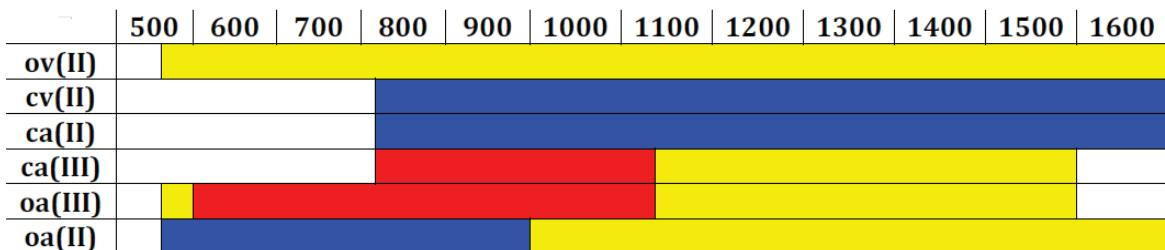
**Figure 25.** Nonlinear behavior of **79** across its six states as a function of the laser irradiation wavelength (nm, horizontal scale). **o** = open form, **c** = closed form, **a** = alkynyl, **v** = vinylidene, (II/III) = formal oxidation state of the metal centers. Red: saturable absorber, blue: nonlinear absorber, yellow: inactive nonlinear absorber, white = no data reported [70].
