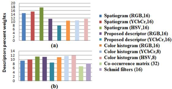
Figure 3: Descriptors percent weights: (a) color descriptors cascade (b) color and texture descriptors cascade.
