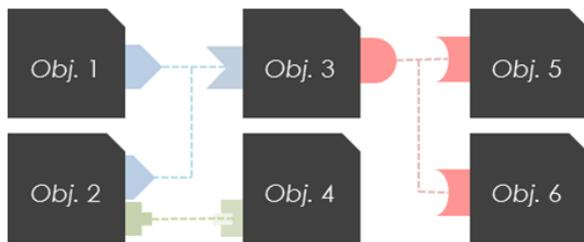
Fig. 10 A BeC<sup>3</sup> application where multiple objects interact. If outputs match correctly needs and conversely, the Choreography may be deployed and started.
