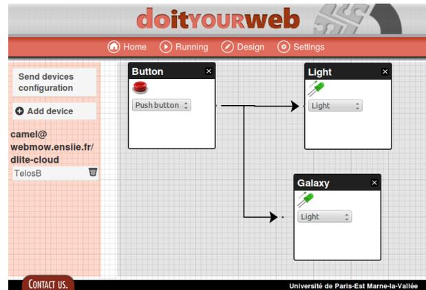
**Fig. 13** The Design screen of *BeC<sup>3</sup>* mashup tool, showing all devices. The *behaviour* chosen for each of them is indicated on the option list field. Publish-subscribe relations are shown with arrows. One node (TelosB) is available (on the left). Application is deployed with "Send devices configuration".
