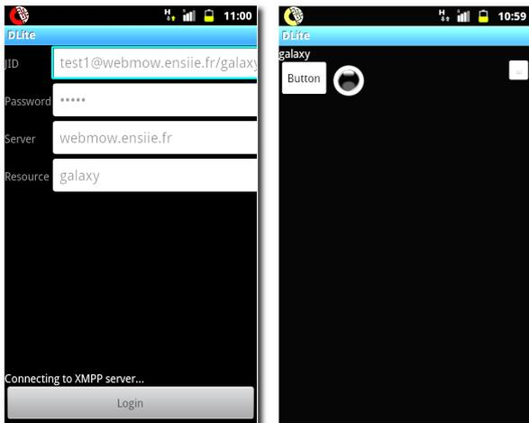
**Fig. 12** D-LITE for Android. After authentication screen (on the left) that helps the identification of the device, the smartphone receives the logic it has to execute. In this example, this node has been remotely configured to offer a button and a pseudo-led that can be switched on or off by other nodes, according to *BeC<sup>3</sup>* uploaded logic (right screen).
