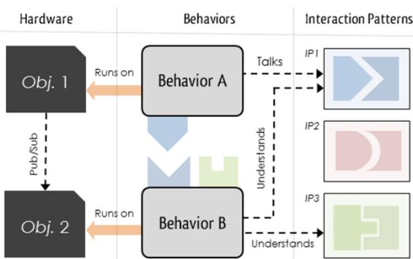
Fig. 9 Two Objects running BeC<sup>3</sup> Behaviours. They interact because the two Behaviours correctly match the required Interaction Patterns. Object 2 runs a Behaviour that “understands” IP1 (needs it as an input), and optionally IP3. Object 1 runs a Behaviour that “talks” IP1. So publish/subscribe can be done.
