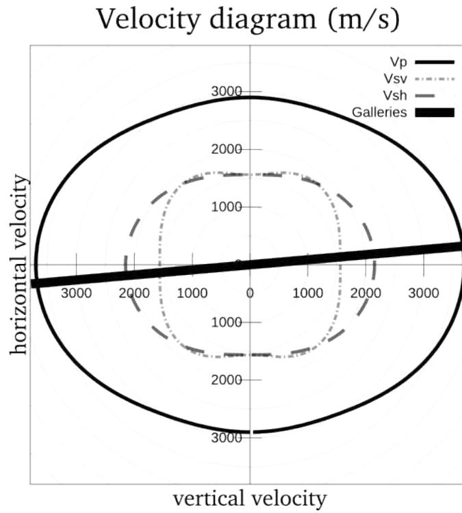
Figure 3: Anisotropy diagram computed using Thomsen's parameters (Thomsen, 1986) estimated by Zinszner et al. (2002) and velocities estimated in the preliminary studies. The thick black line represent the relative inclination of the galleries compared to the stratification plane in the most unfavorable configuration ( $5^\circ$ ).
