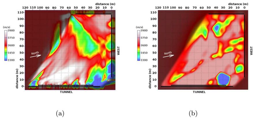
Figure 16: Velocity maps obtained from the experimental data with (a) traveltime tomography (b) damped robust acoustic full waveform inversion.
