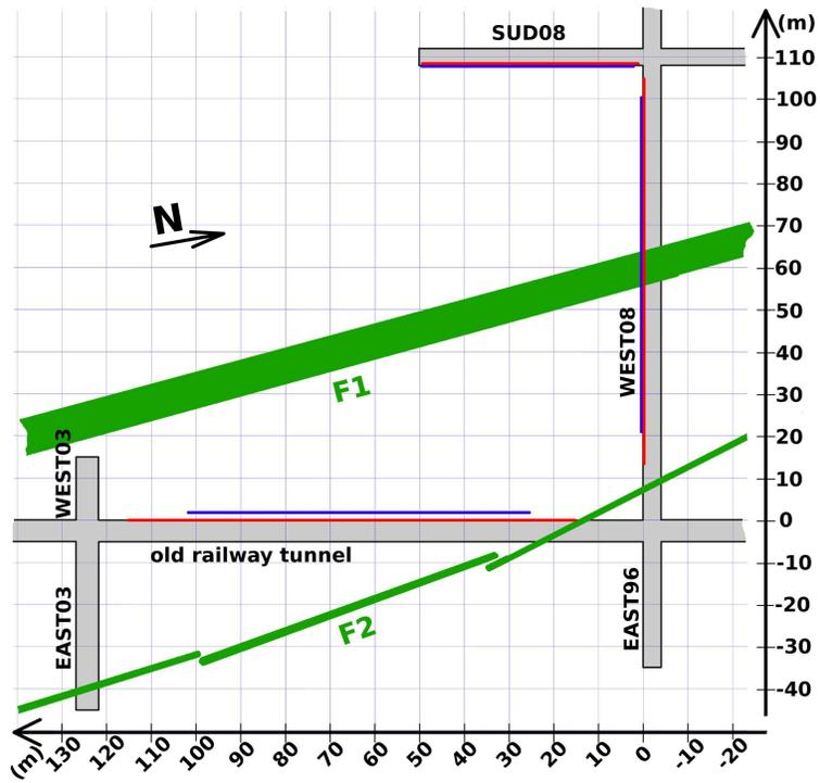
Figure 2: Map of the central zone of the TEP showing underground works and fault zones F1 and F2 at their location (green) expected from visual inspection of galleries and from information in boreholes. The positions of sources and receivers respectively represented in red and blue delimit the investigated area.
