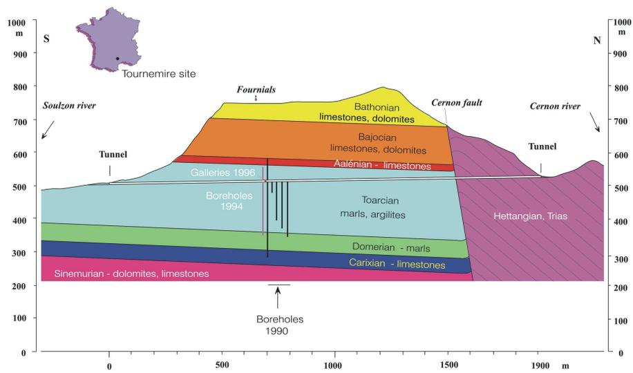
Figure 1: Geological cross-section of the Tournemire site along the tunnel of the TEP. The galleries are located in the central part of the TEP.
