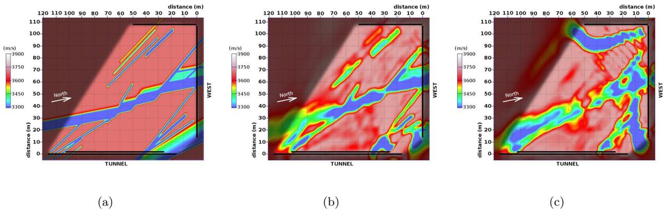
Figure 19: Velocity maps obtained in the synthetic interpreted model. (a) exact interpreted model, final inverted models at 600 Hz from (b) damped acoustic inversion of acoustic data (c) damped acoustic inversion of elastic data.
