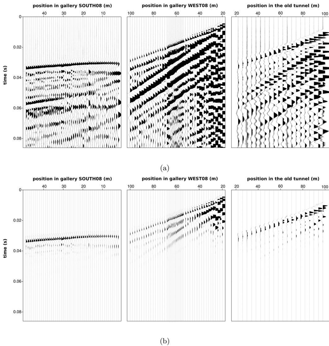
Figure 12: Examples of common shot gathers from the old railway tunnel:(a) Raw data (b) data after application of the time domain damping  $e^{\gamma(t-t_0)}$ .
