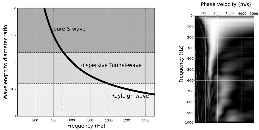
Figure 4: Impact of the gallery on shear waves propagating along the galleries. (a) wavelengths to diameter ratio versus frequency and behavior limits according to Jetschny et al. (2010). (b) Rayleigh wave dispersion diagram computed from preliminary seismic data recorded in the undisturbed rock in gallery WEST08.
