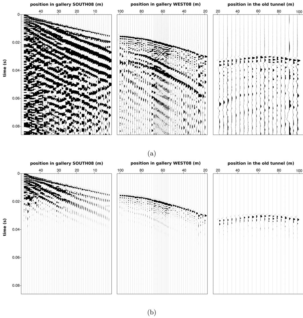
Figure 11: Examples of common shot gathers from the gallery SOUTH08: (a) Raw data (b) data after application of the time domain damping  $e^{\gamma(t-t_0)}$ .
