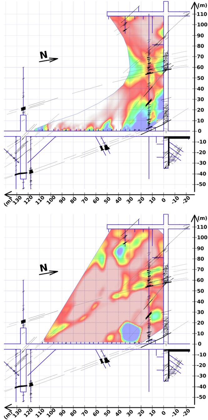
Figure 17: Velocity maps obtained from the experimental data with (a) traveltime tomography (b) damped robust acoustic full waveform inversion, both presented with location of fault zones and fractured areas (black) mapped from observations in galleries and bore-holes (blue) (Cabrera, 2013). Gray lines give locations of faults and fractures locations extrapolation from the real observed structures.
