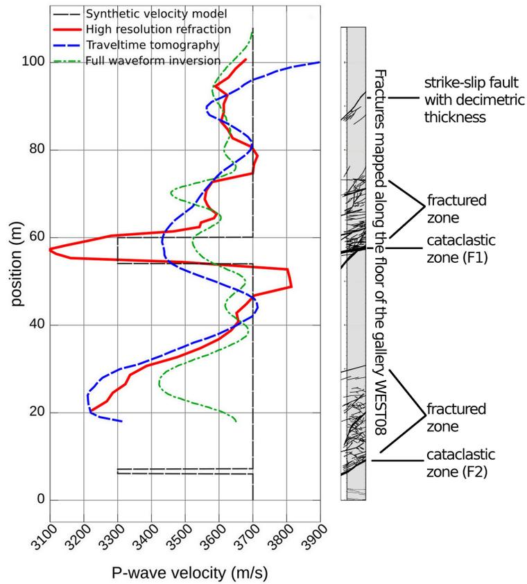
Figure 18: Fractures mapping and velocity profiles along the gallery WEST08 (1 m from the gallery) from tomography and FWI compared to the high resolution velocity profile obtained with seismic refraction.
