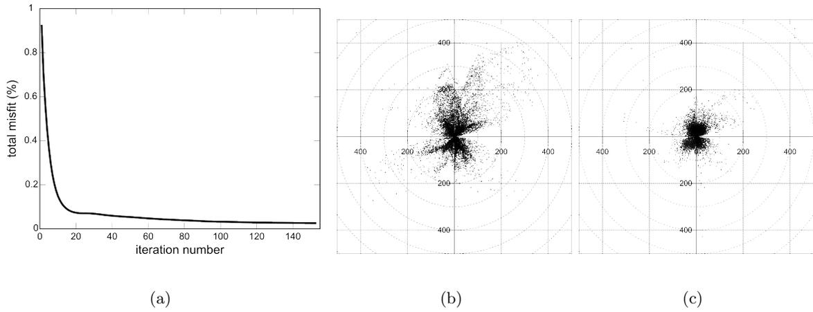
Figure 13: (a) Decrease of the total misfit (b-c) repartition of the average velocity misfit for each ray between experimental data and data computed from homogeneous initial model (b) and model obtained after 150 iteration (c).
