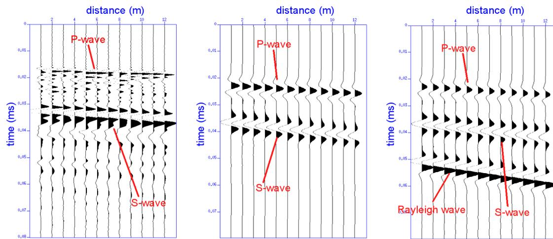
Figure 5: Effect of the galleries on shear waves : (a) experimental shot gather, (b) synthetic shot gather computed with absorbing boundary conditions and (c) with infinite free surfaces.
