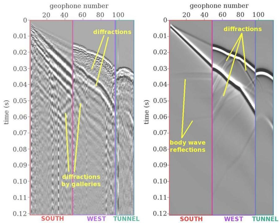
Figure 7: Synthetic and experimental shot gathers: source at the extremity of gallery SOUTH08, receivers respectively in gallery SOUTH08, WEST08 and in the old tunnel.
