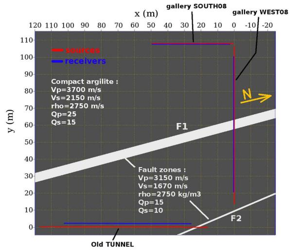
Figure 6: Velocity model of the investigated area used for numerical modeling. The model includes viscoelastic parameters of the compact argillite (black) and the F1 and F2 fault zones (white). It is extended to the north to include large offset reflections from gallery SOUTH08, and then extend with PML absorbing layers. Source and receiver positions along the galleries are represented in blue and red.
