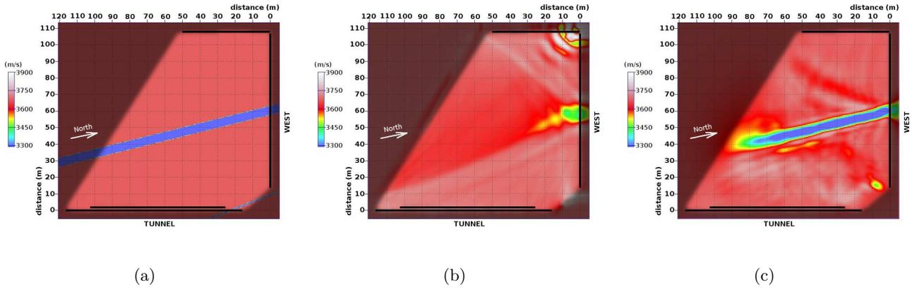
Figure 8: 2D velocity maps obtained by tomographic and waveform inversion of synthetic data: (a) exact model used to compute traveltimes and full waveform data, (b) model obtained with first arrival travel time tomography (c) model obtained with acoustic full waveform inversion.
