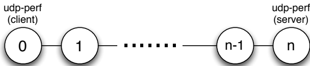
Figure 2: Experimental topology to estimate packet processing rate.
