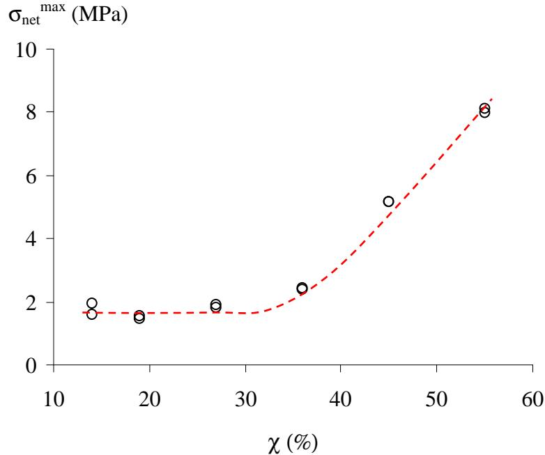
Figure 3.  $\sigma_{net}^{max}$  as a function of the degree of crystallinity  $\chi$  (%)
