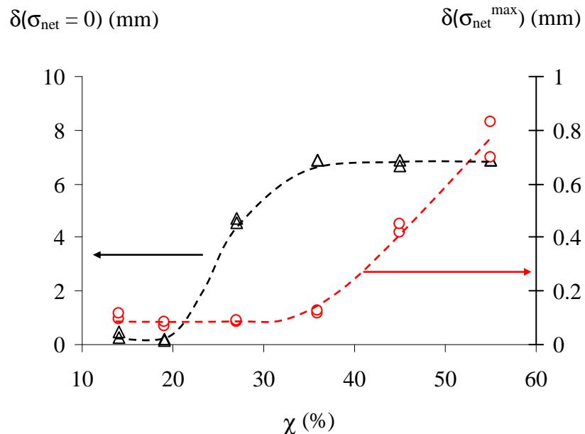
Figure 4.  $\delta(\sigma_{net}^{max})$  and  $\delta(\sigma_{net} = 0)$  as a function of the degree of crystallinity  $\chi$  (%)
