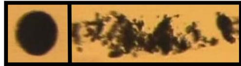
**Figure 3:** illustration of the fragmentation mechanism for a silica agglomerate with an initial radius of 37  $\mu\text{m}$  at 56s<sup>-1</sup>
