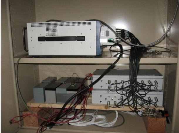
Figure 38 Picture of the DAC in its Faraday cage
