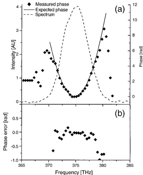
Fig. 4. (a) Diamonds, difference in spectral phase between two time-domain HOT SPIDER measurements that differ by a known amount of second-order phase ( $8300 \text{ fs}^2$ ). The expected spectral-phase difference and the spectral intensity (spectrum) are also shown. (b) Phase error computed by subtraction of the theoretical phase from the measured value.
