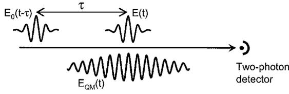
Fig. 2. Time-domain HOT SPIDER. The second-order nonlinear signal is recorded by a two-photon time-integrating detector as a function of time delay  $\tau$  between a reference pulse,  $E_0$ , and a superposition of two pulses: the pulse to be measured,  $E$ , and a quasi-monochromatic pulse,  $E_{QM}$ .
