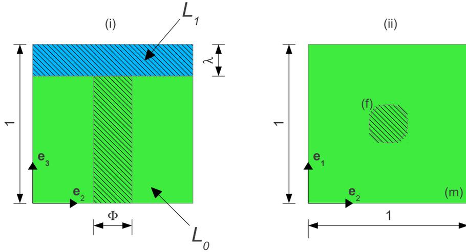
Figure 1: Unit-cell of 2-1-2 periodic composites with homogeneous layers  $L_1$  (blue) and heterogeneous layers  $L_0$  (green) made of a matrix phase (m) and aligned fibers (f) with a regular square distribution in the cross-section. The fibers (f) and the layers  $L_1$  are made with the same material (hatched area). Left: longitudinal cut of the unit cell. Right: bottom-view of the unit cell.
