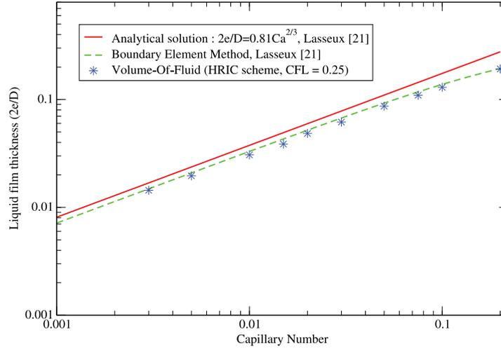
**Fig. 3.** Dimensionless liquid film thickness as a function of capillary number during the drainage of a liquid phase in a vertical tube. Comparison between VOF simulation and a reference solution (Lasseux [21]).
