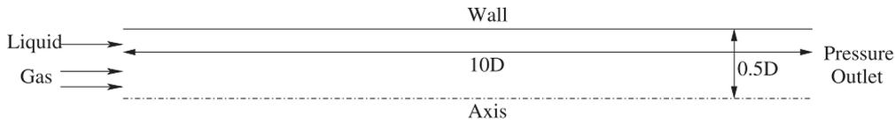
**Fig. 10.** Geometry and boundary conditions for the Taylor bubbles simulations.**Table 4**
