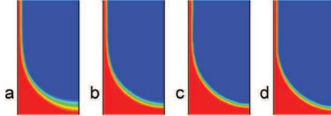
**Fig. 9.** A comparison of the interface dissipation from the less to the most compressive scheme ( $Co = 0.25$ ,  $Ca = 0.03$ ), (a) QUICK, (b) HRIC, (c) CICSAM, (d) Geo-Reconstruct.
