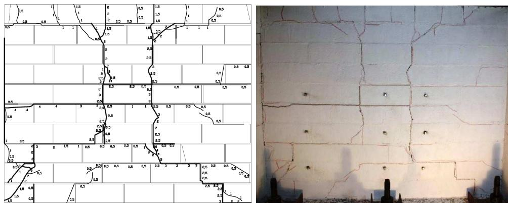
**Figure 9.** Wall 2- Failure modes of the principal wall
