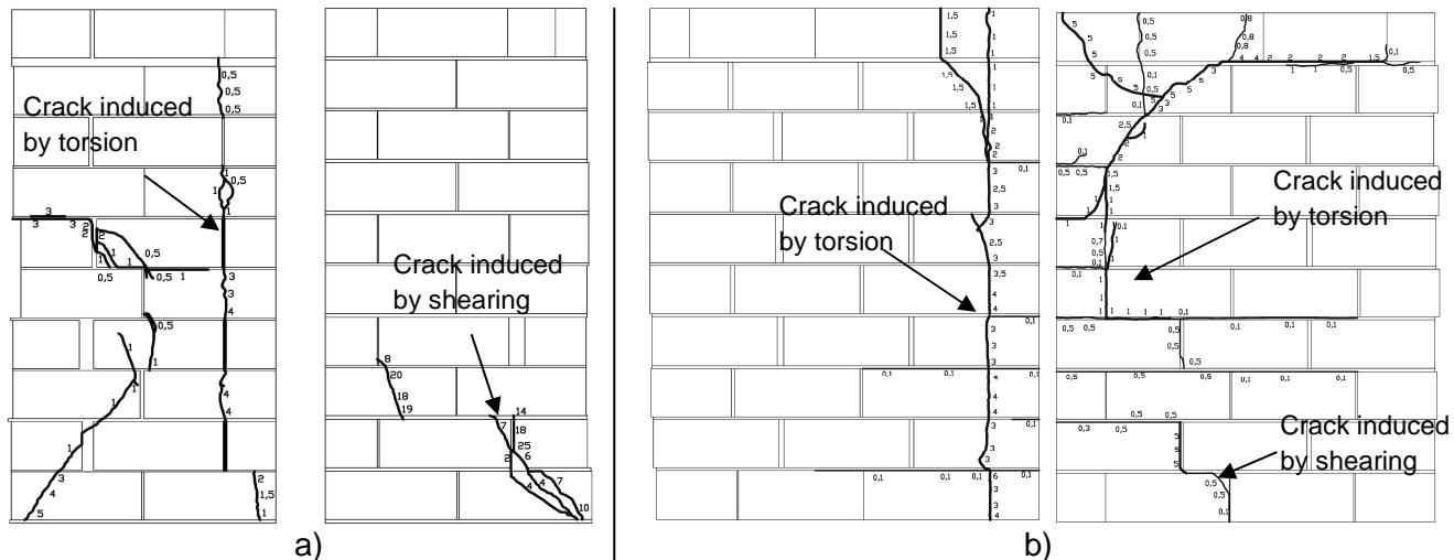
**Figure 10.** Failure modes of the two return walls: a)Wall 1; b)Wall 2
