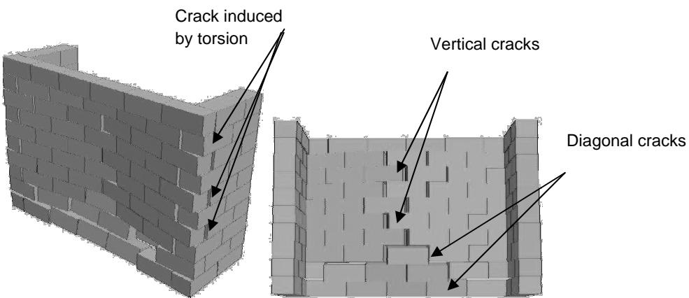
**Figure 14.** The cracking pattern obtained numerically
