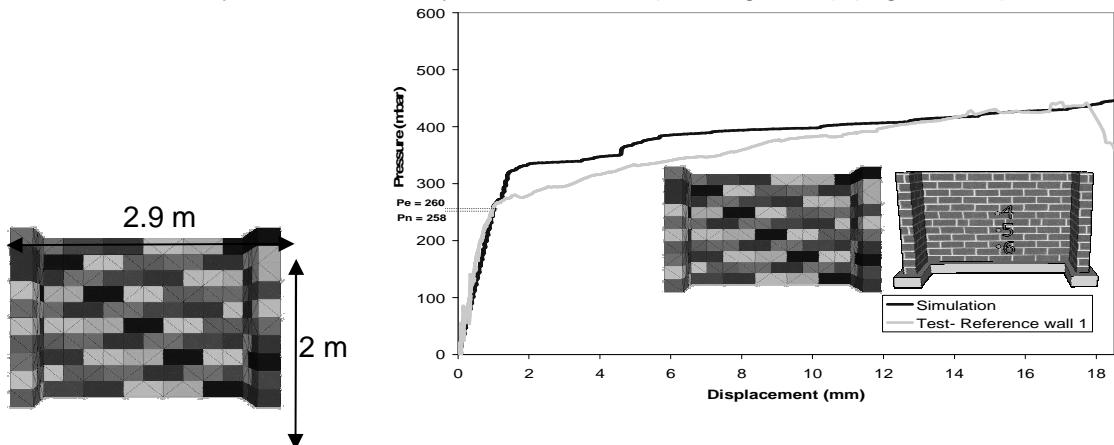
**Figure 13.** a) Complete mesh ; b) Pressure/deflection curve: comparison test/calculation
