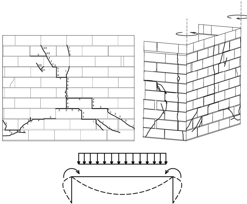
**Figure 8.** Wall 1- Failure modes of the principal wall
