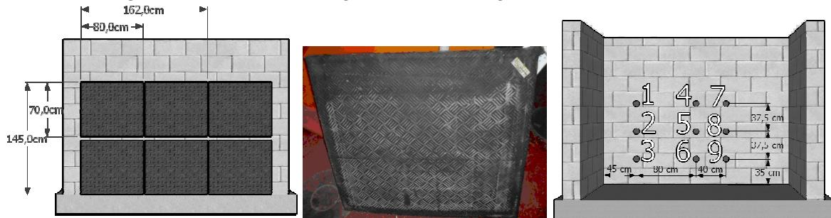
**Figure 3.** Water-bags on the north side and transducers positioned on the south side of the wall.
