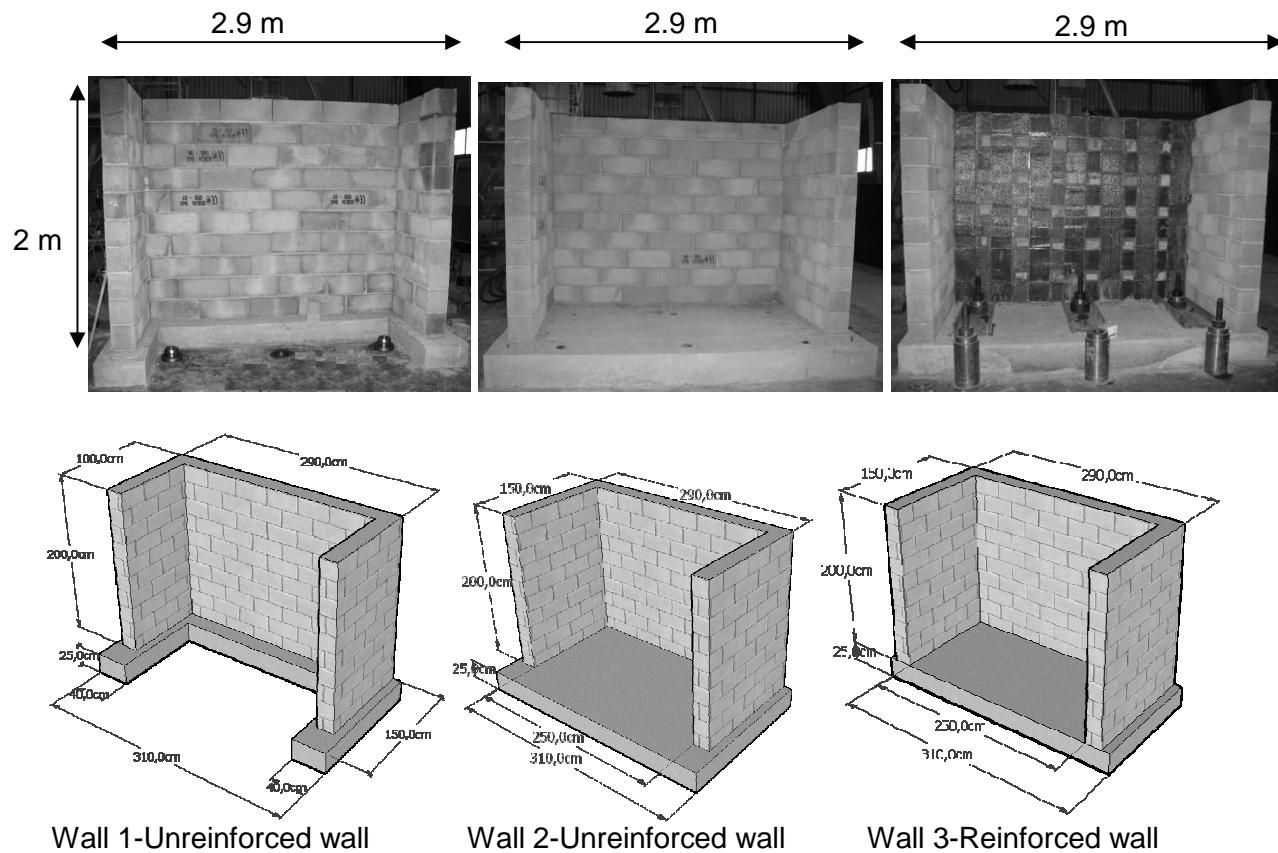
**Figure 1.** Unreinforced (wall 1 & 2) and reinforced masonry wall (wall 3). Specimens 1, 2 and 3
