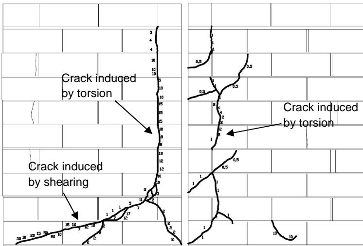
**Figure 12.** Wall 3 – Failure modes of the two return walls
