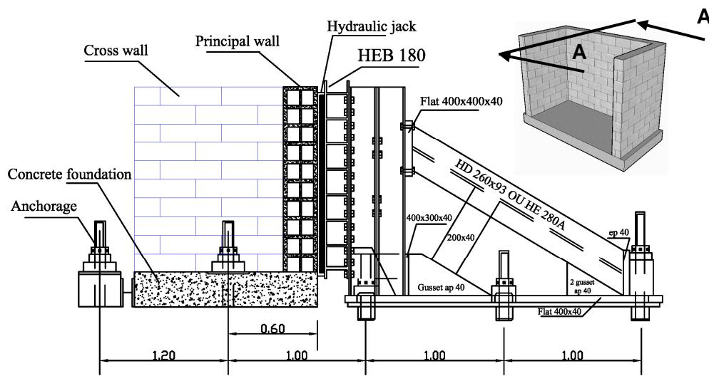
**Figure 2.** Laboratory test arrangement according to section AA.
