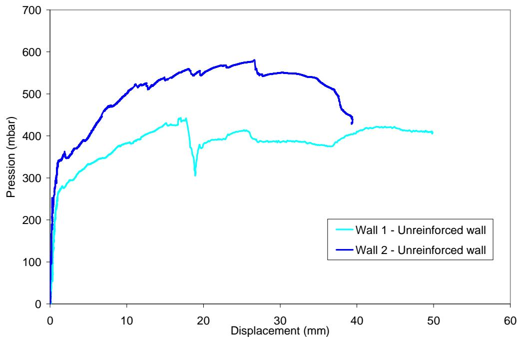
**Figure 5.** Comparison between two unreinforced walls
