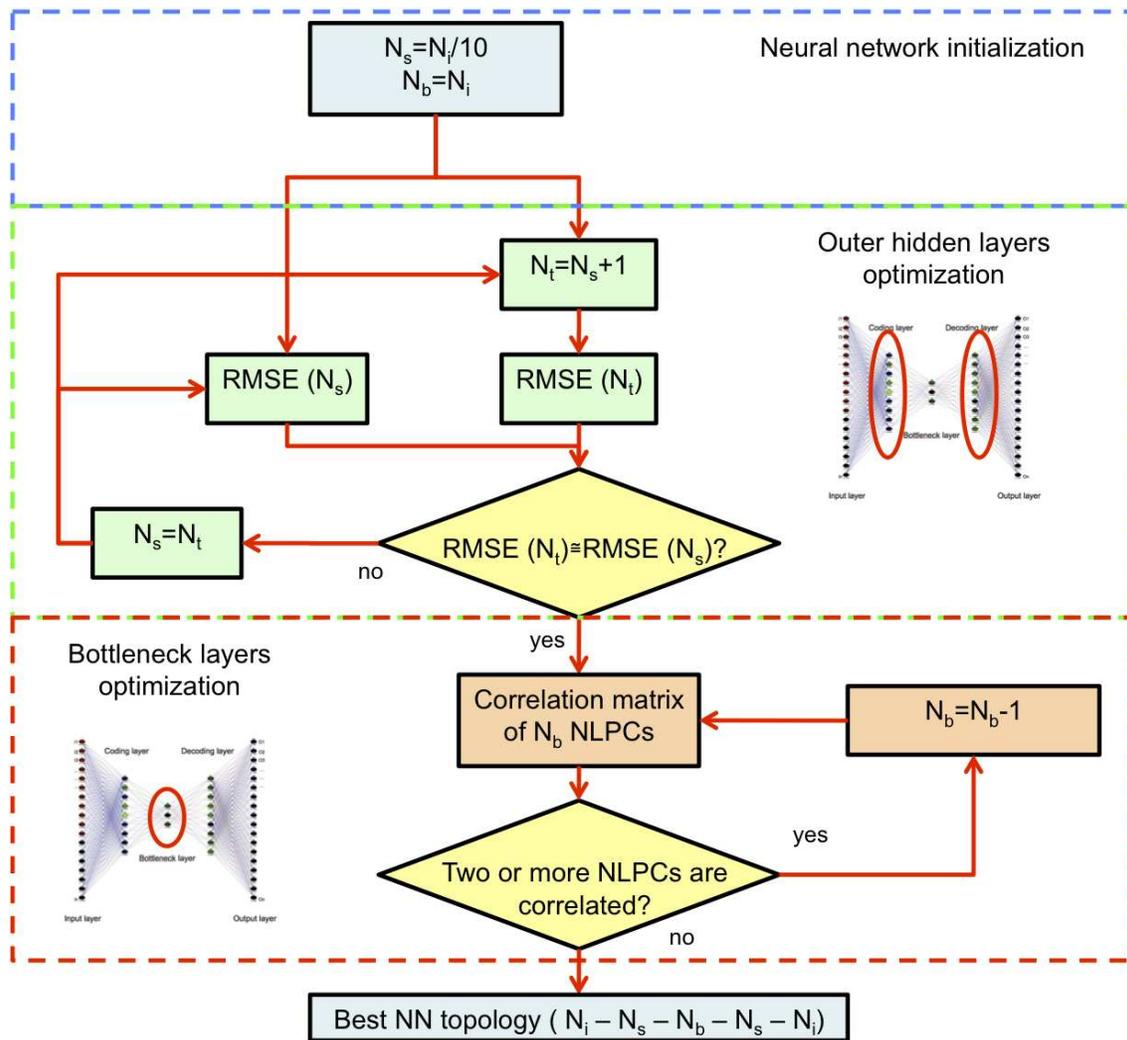
**Fig. 5.** Complete flowchart describing the optimization of the topology of the AANN.  $N_i$ ,  $N_s$  and  $N_b$  represent the number of nodes in the input/output, in the outer hidden layers and in the bottleneck layer, respectively.
