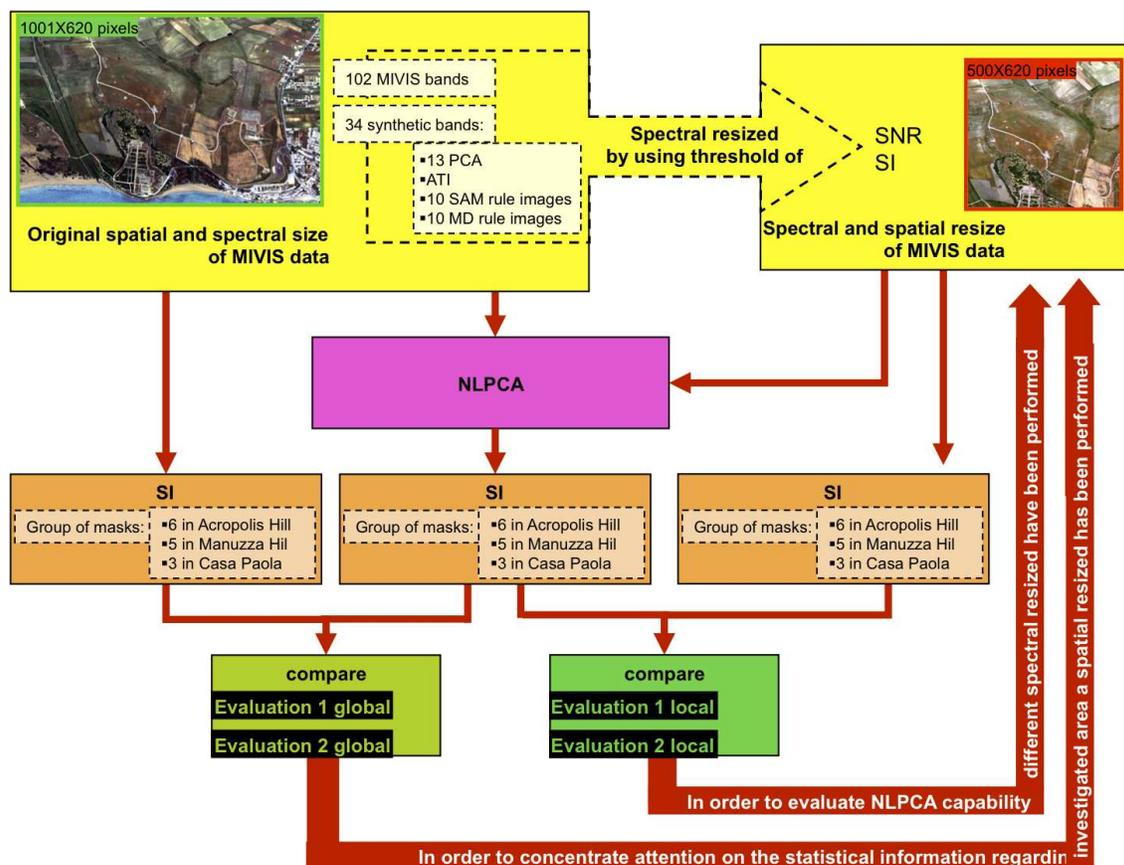
**Fig. 9.** Flowchart of the process carried out to evaluate the potentiality of NLPCA to produce features able to emphasize the anomalies related to the presence of buried structures. The two RGB images are referred to the original spatial size of the MIVIS data (left) and the resized one (right).
