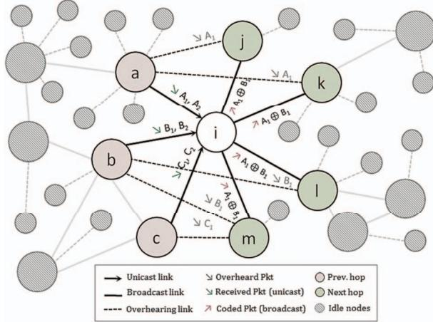
Figure 1 - ZigBee overhearing example
