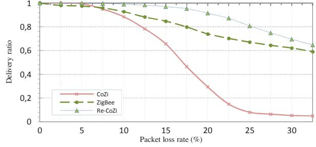
Figure 3 – Delivery ratio versus packet loss rate
