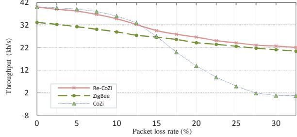
Figure 5 – Throughput versus packet loss rate
