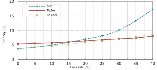
Figure 4 – Latency versus packet loss rate
