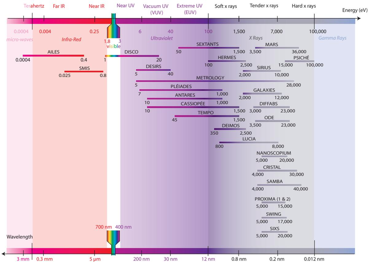
Figure 7.2: This scheme shows the photon energy range covered by the beamlines installed at the SOLEIL synchrotron facility [17]. The TEMPO beamline stands in the UV-Soft X-rays range.
