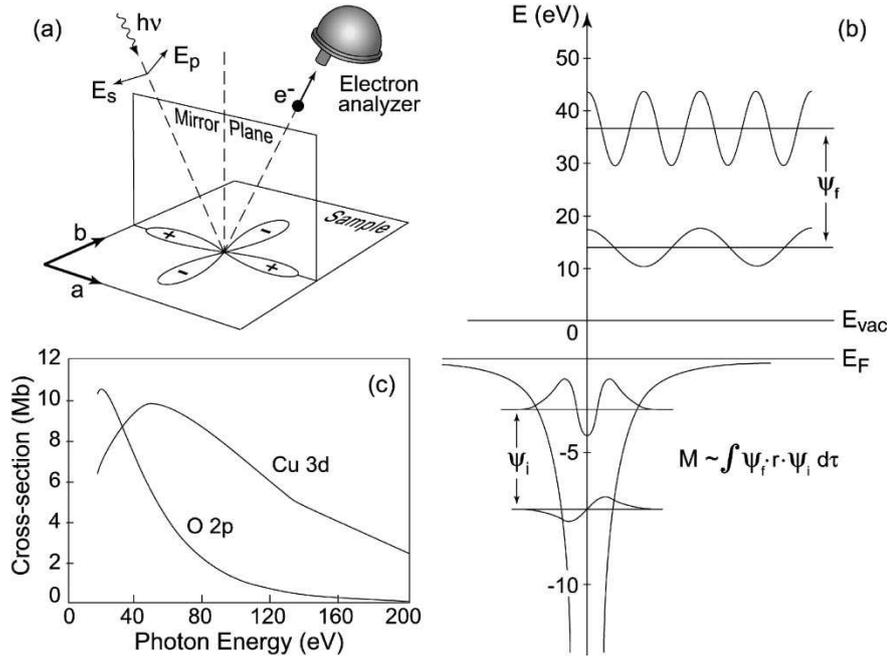
Figure 3.4: (a) Sketch of a photoemission experiment. The figure shows how polarization and wavefunction parity are connected with the experimental setup. In this example a  $d$ -type orbital of even parity is sketched. (b) Schematic example of an optical transition between atomic orbitals with different momenta. (c) Example of photo-ionization cross sections for Cu 3d and O 2p atomic orbitals [83]. Image taken from [6].
