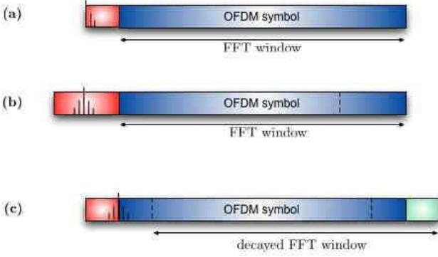
Fig. 7. Guard interval design and associated synchronization for classical CP-OFDM (a), TR-OFDM with a double CP (b) and TR-OFDM with CP and CS (c)
