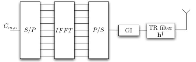
Fig. 2. OFDM transmitter including a Time Reversal filter
