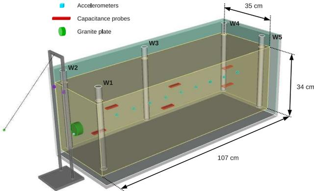
**Figure 2.** Schematic view of the experimental set-up. A steel ball mounted on a pendulum hits a circular granite plate on the left lateral side of the sand-filled tank. Wave propagation is monitored by nine aligned buried accelerometers. Water saturation level is measured by capacitance probes. Five wells W1-W5 are used to proceed to imbibition or drainage.
