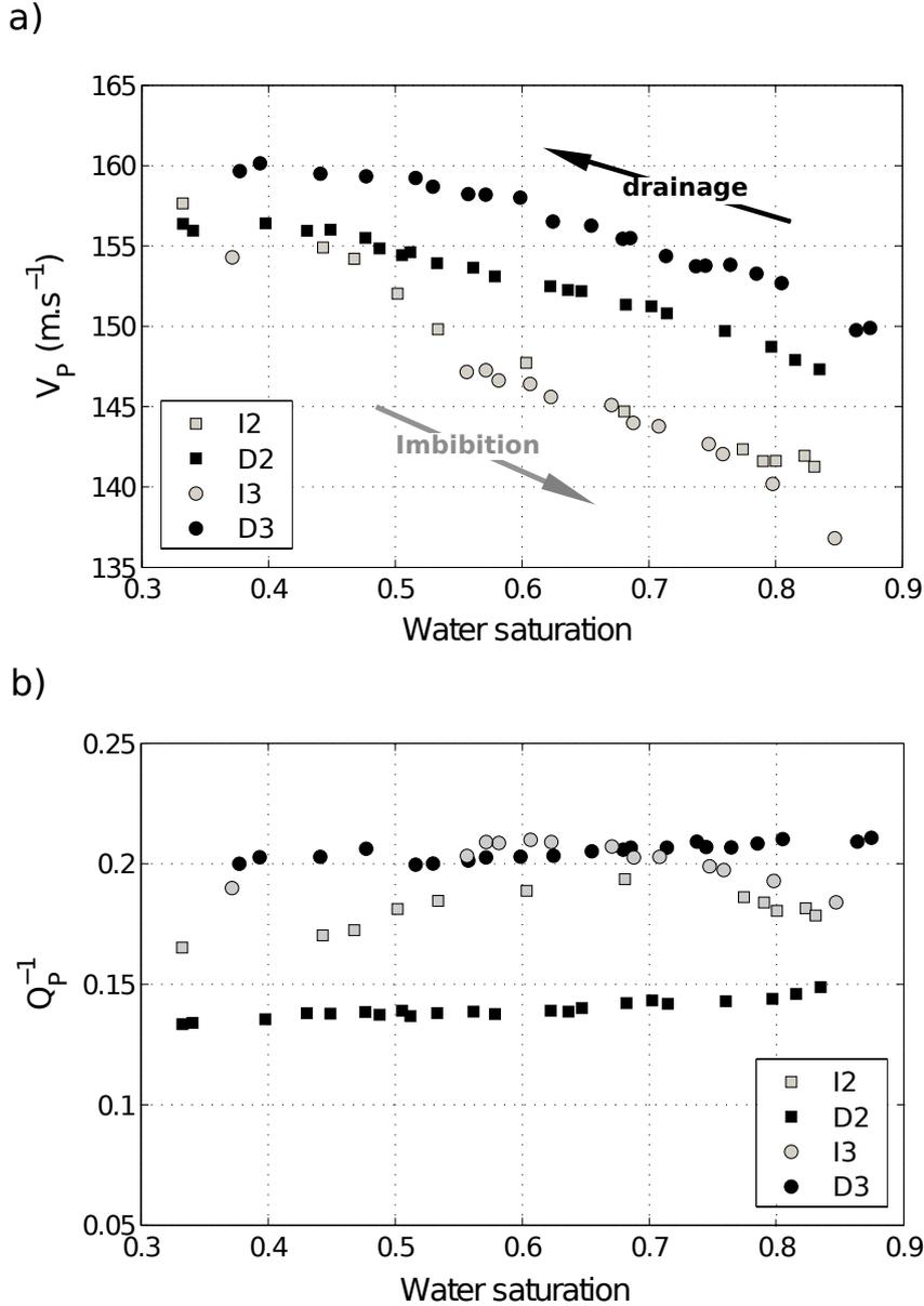
**Figure 6.** a) Measured P-waves phase velocity  $V_P$  and b) inverse quality factor  $Q_P^{-1}$  as a function of  $S_w$ , recorded during the second imbibition I2, the second drainage D2, the third imbibition I3 and the third drainage D3, for  $f = [1.6 - 1.8]$  kHz. The arrows in a) indicates that imbibition results in increasing  $S_w$  in time whereas drainage results in decreasing  $S_w$ . The experimental error-bars at each data point are shown in Figure 7.
