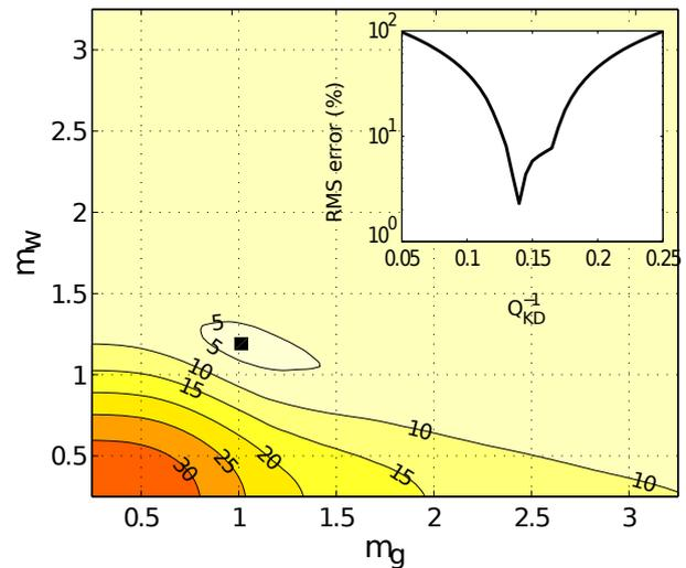
**Figure 8.** Least-square inversion residuals for  $Q_{KD}^{-1}$ , and least-square inversion residuals maps ( $m_g, m_w$ ) for the best  $Q_{KD}^{-1}$ . The residuals are shown for the experiment I2, D2, I3, D3 in a), b), c) and d) respectively. The effective pressure is varying for I2 and I3 in a) and c), and is constant for D2 and D3 in b) and d) (see Table 3).
