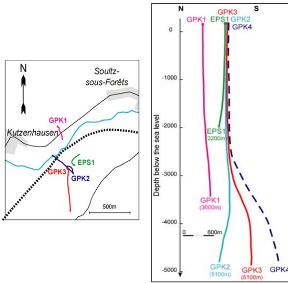
Figure 2a - Location map and profiles of the geothermal wells (from Gentier *et al.*, 2003a and b).
