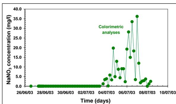
Figure 5 - Geochemical monitoring of the fluid discharged from the well GPK-2 (from 26/06 to 9/07/2003): Analytical results of the NaNO<sub>3</sub> tracer obtained using the colorimetric technique on site.
