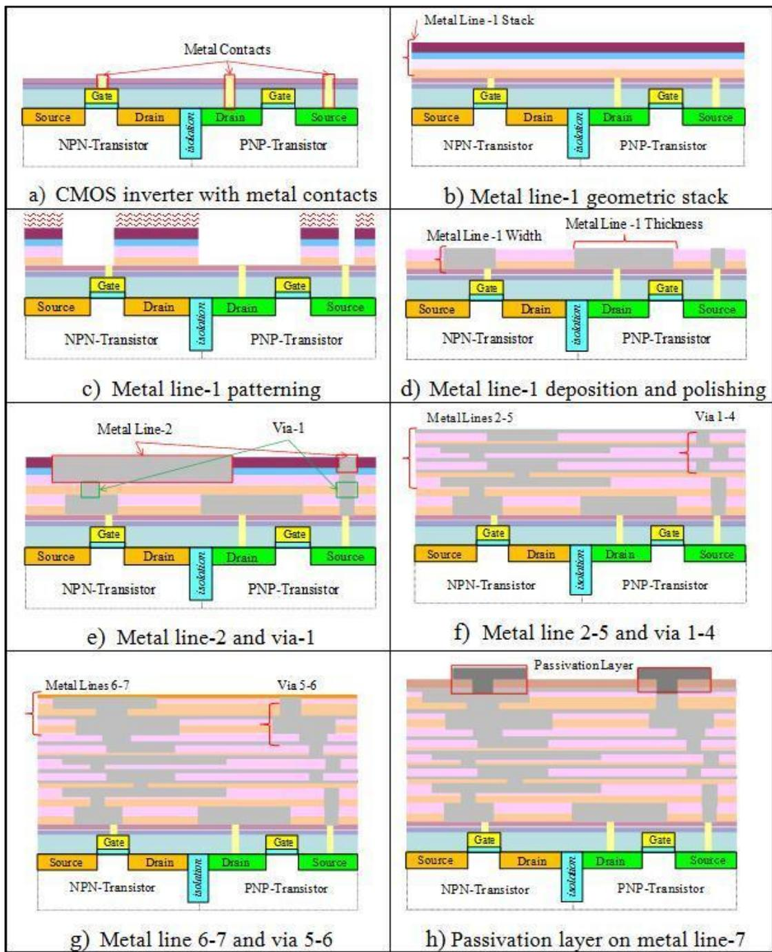
Figure 5.7 – The BEOL – process for interconnections
