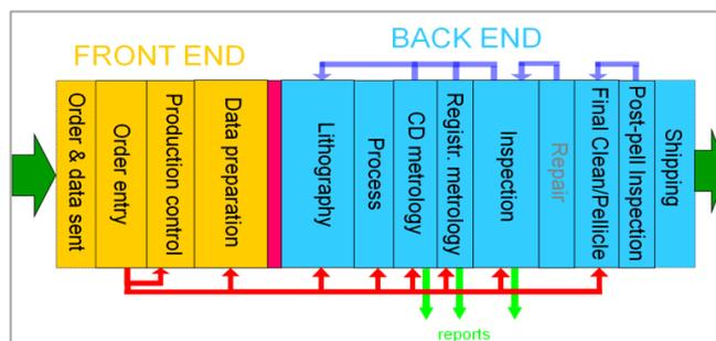
Figure B.5 - mask fabrication flow
