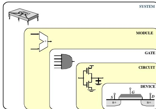
Figure B.2 – Reusability and modularity concept in electronics circuits
