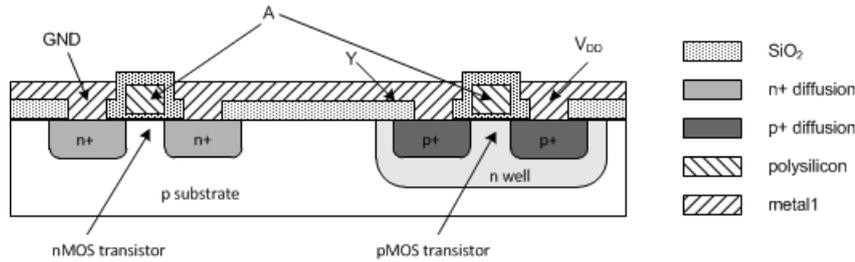
Figure C.10 – CMOS inverter’s structural cross section view
