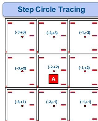
Figure 5.24 – The example of basic step-circle algorithm (step-2)
