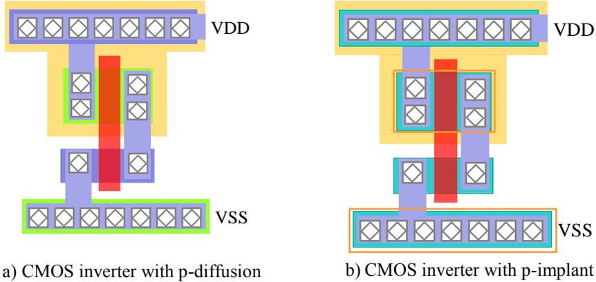
Figure C.6 – Physical design of CMOS inverter [Lee, 2005]
