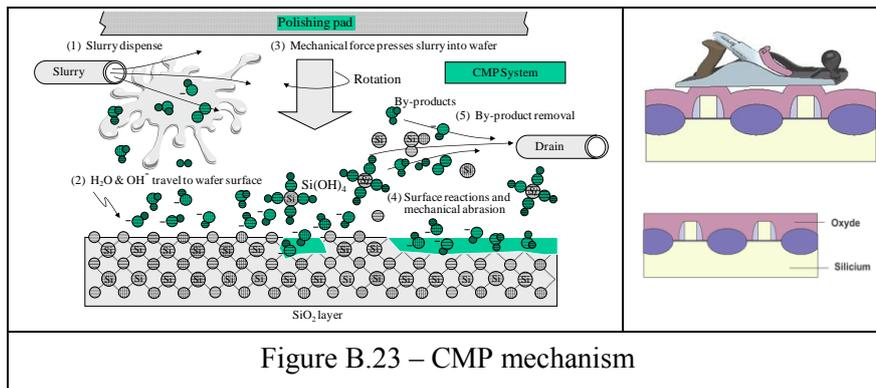
Figure B.23 – CMP mechanism
