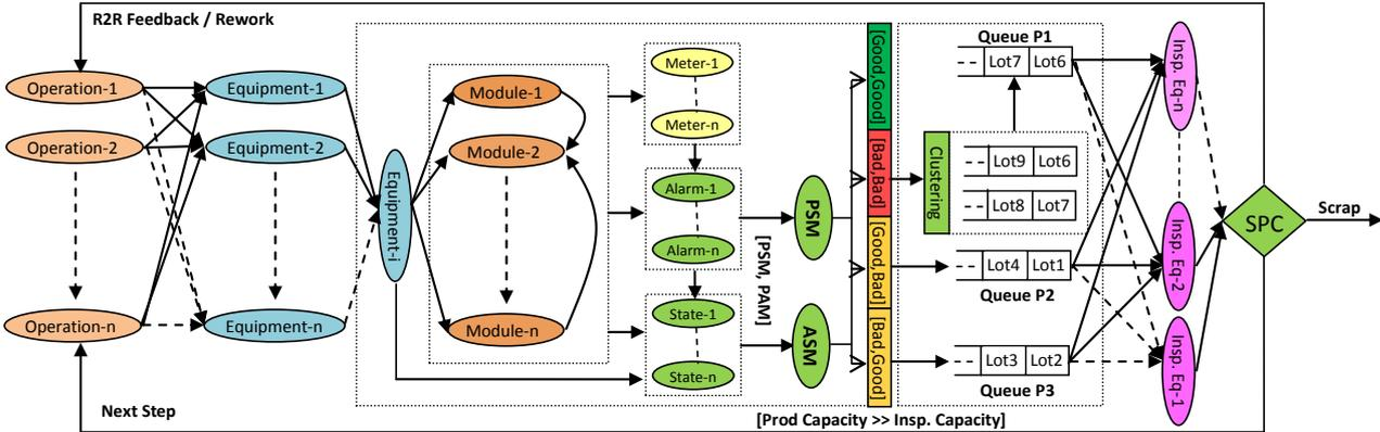
Figure 7.2 - Methodology with predictive state (PSM) and alarm (PAM) models
