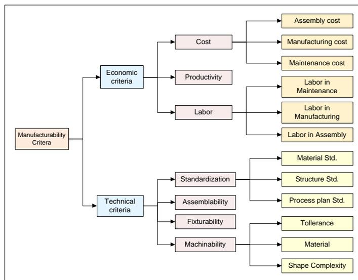
Figure 2.14 - Manufacturability criteria for IC designs [Yuyin et al., 1996]
