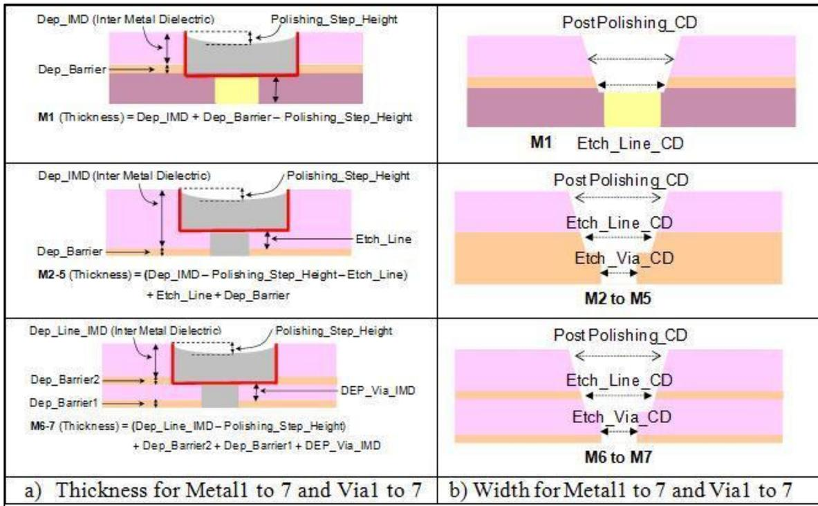
Figure 5.8 – The BEOL – geometric computations in BEOL process
