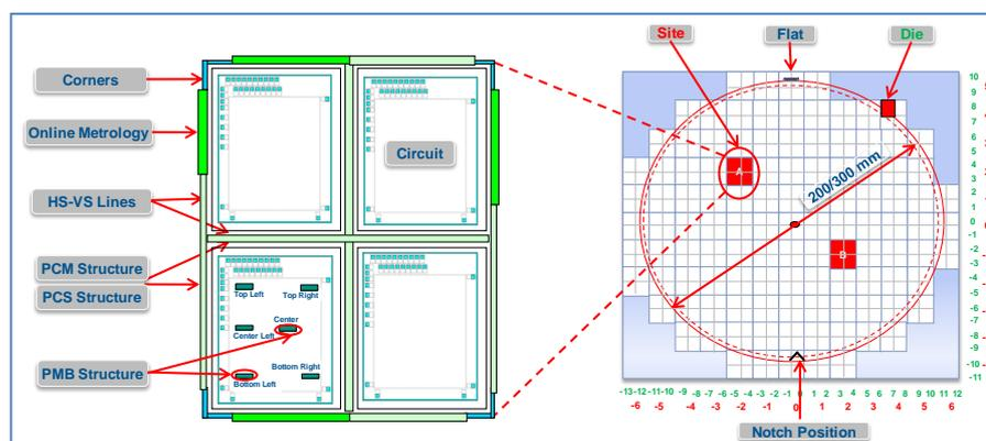
Figure 5.21 – Structure of wafer, sites and dies
