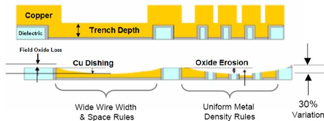
Figure B.24 – Dishing and erosion mechanisms.
