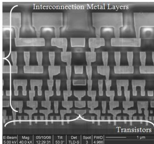
Figure 1.5 - Cross section of an electronic chip (transistors and interconnects)
