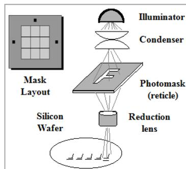
Figure B.4 - The mask layout and its use in photolithography
