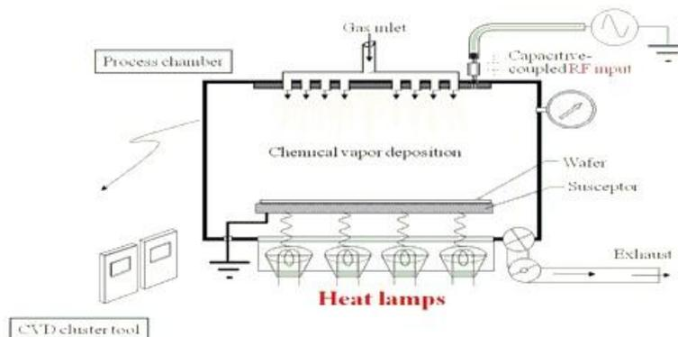
Figure B.22 – Structural description of the CVD process.
