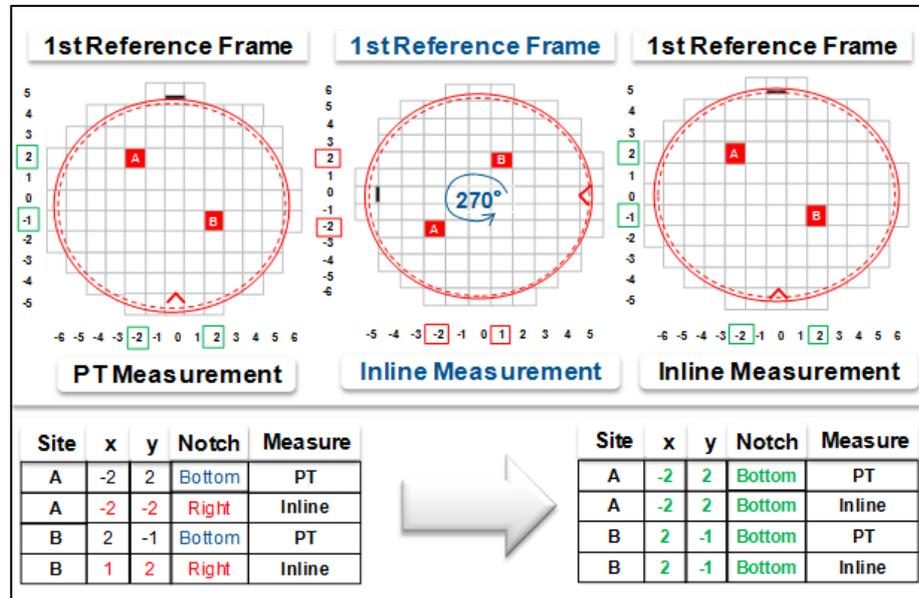
Figure 5.10 – Site/Site level mismatches due to notch position
