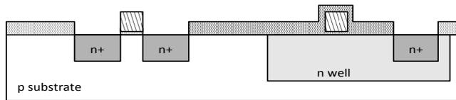
c) n+ diffusion and source, drain and n-well contact
