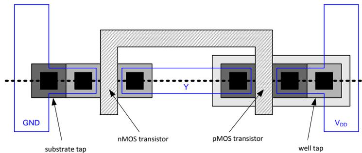
b) Combined masks and resulting CMOS inverter structure
