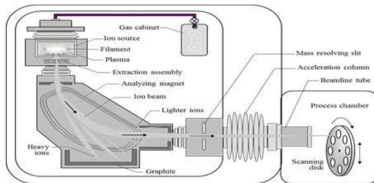
Figure B.21 – Structural description of the Etch process
