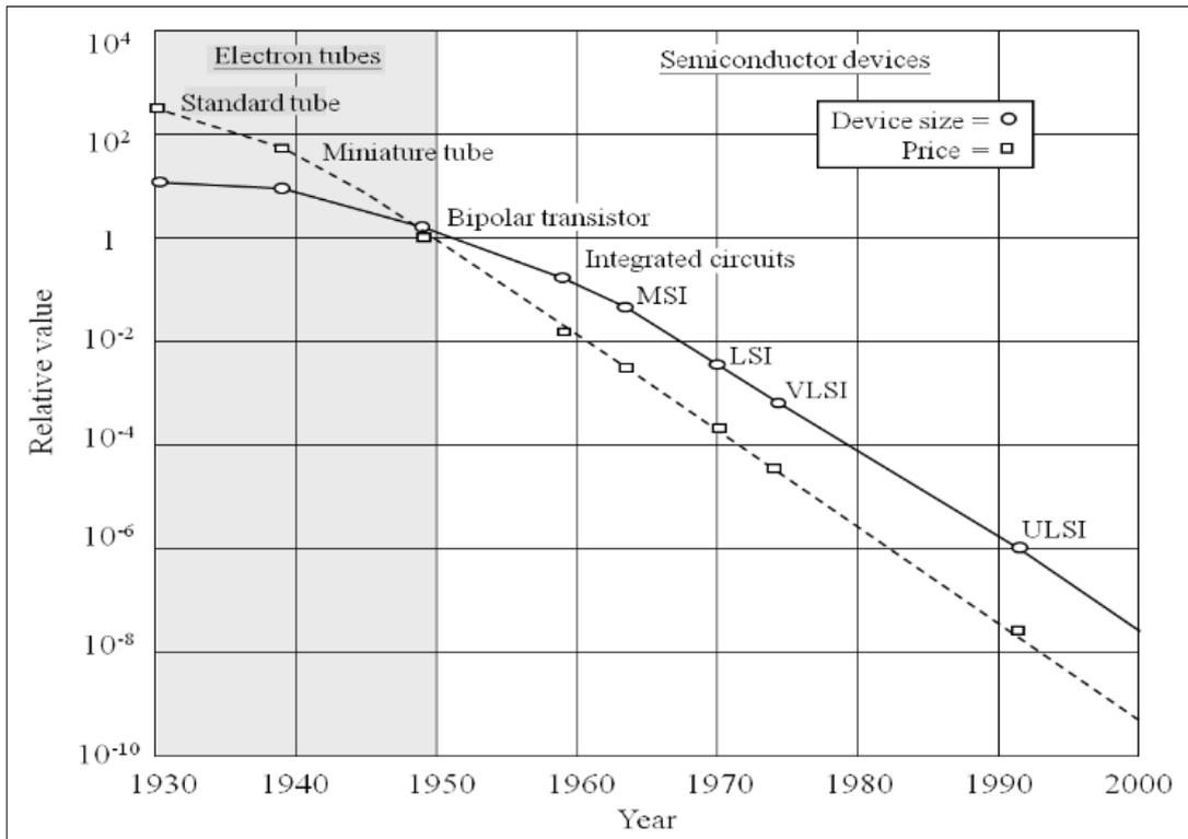
Figure 2.5 – Circuit integration eras and reducing costs (Chang and Sze, 1996)<sup>6</sup>
