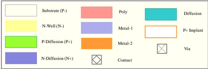
Figure C.5 – Colors and notations for CMOS inverter CAD design
