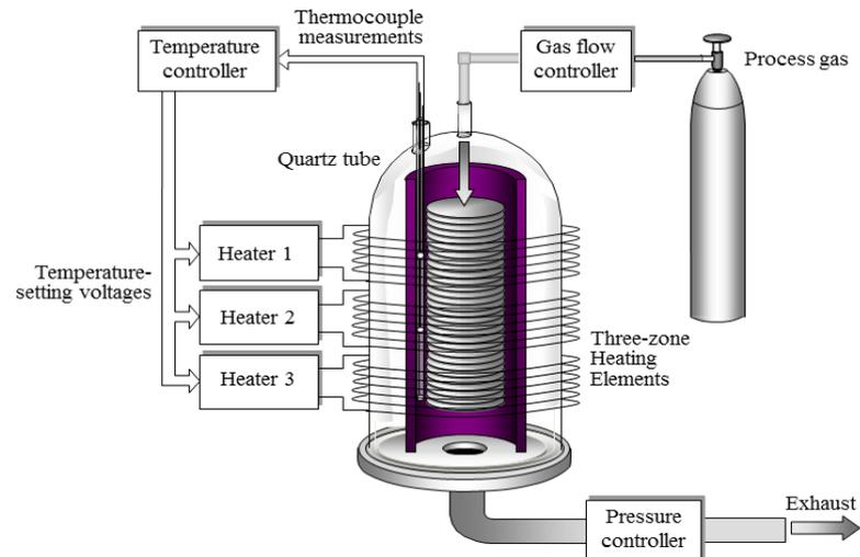
Figure B.18 – Structural description of the oxidation furnace
