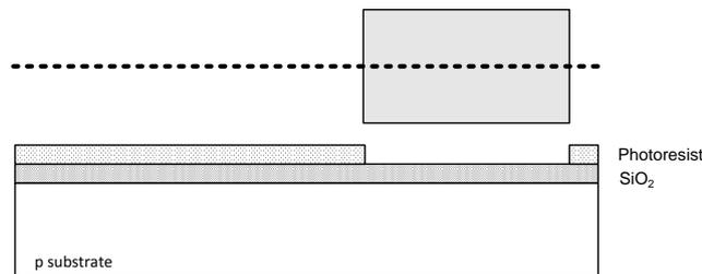
b) n-Well mask is used for the pattern transfer
