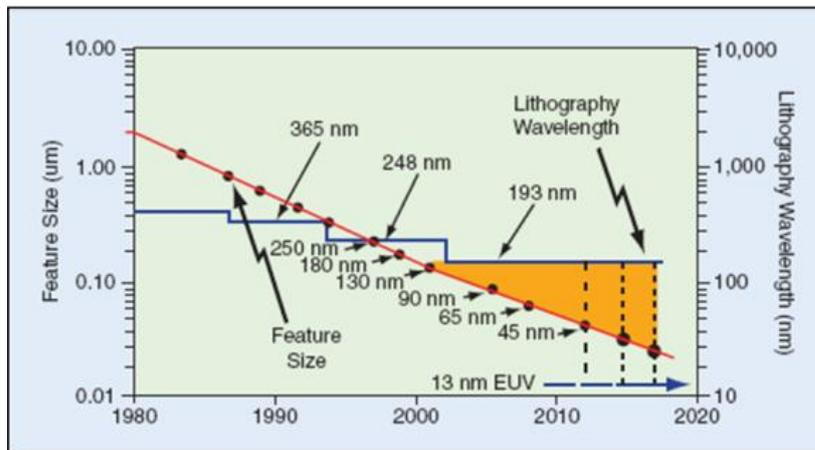
Figure 1.10 - Lithography and feature size [Radojicic et al., 2009]
