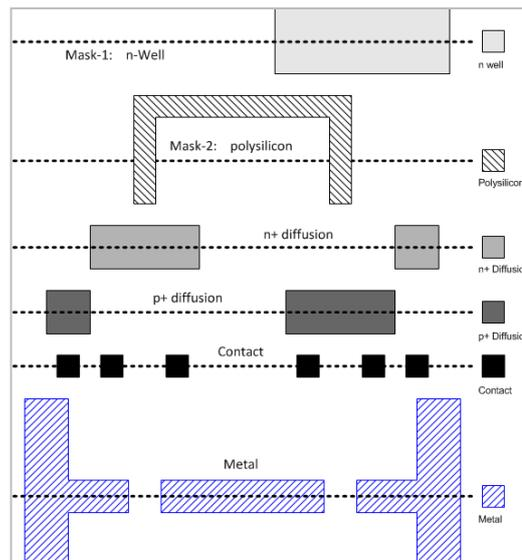
a) Individual masks for CMOS inverter manufacturing
