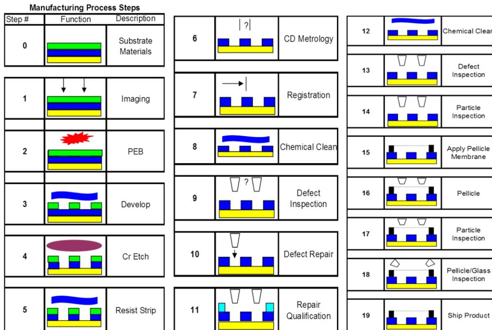
Figure B.7 - back-end mask manufacturing flow
