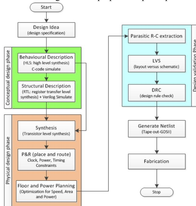
Figure B.3 – Generic design flow for an integrated circuit
