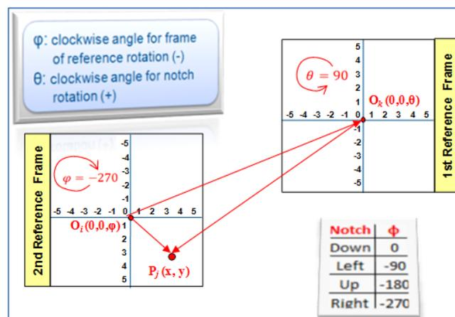
Figure 5.15 – Generic formulation for reference frame and notch position rotation
