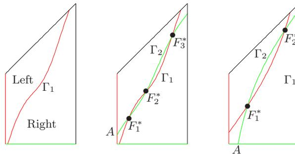
FIGURE 4. On the left, the left and right sides of  $\Gamma_1$ . In the center, the point  $A$  at the very left of  $\Gamma_2$  lies on left side of  $\Gamma_1$ : there are generically an odd number of intersections (3 in this example). On the right, the point  $A$  at the very left of  $\Gamma_2$  lies on right side of  $\Gamma_1$ : there are generically an even number of intersections (2 in this example).
