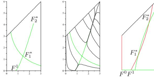
FIGURE 8. Numerical solutions in the bistability case  $D = 0.95$  and parameter values (13). On the left, the separatrix (in green) of the saddle point  $F_1^*$  separate the domain  $\mathcal{S}$  into two regions which are the basins of attraction of the boundary equilibrium point  $F^1$  and the positive equilibrium point  $F_2^*$ . In the center, the phase portrait. On the right, the isoclines.
